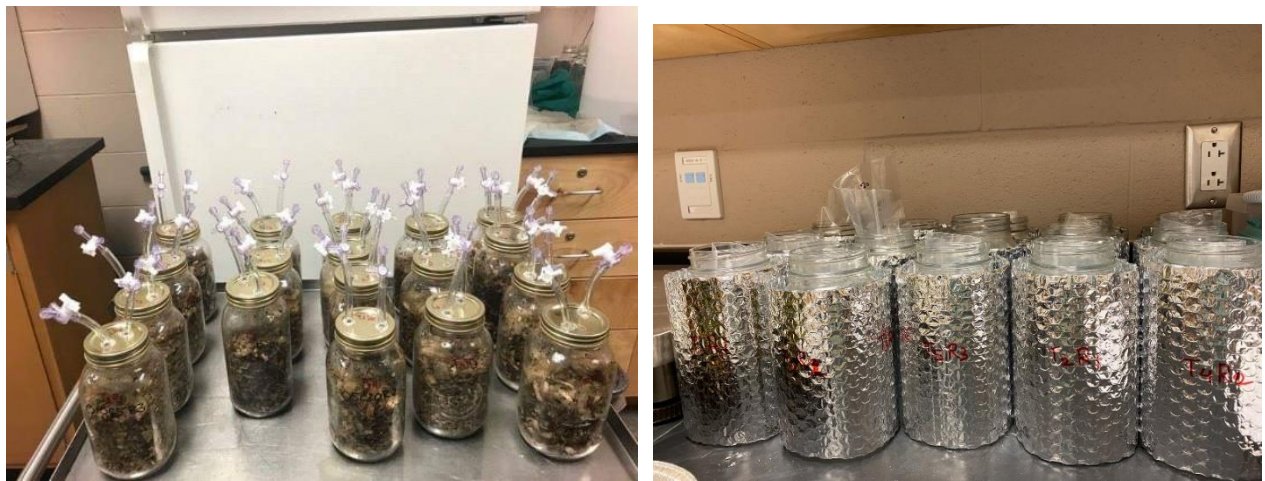
Figure 3.3 Images showing 1 L mason jars filled with composting material with lids prepared for GHG collection (left) and jars covered with insulating materials (right).
