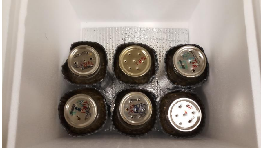
Figure 3.2 Plan images showing 1 L mason jars filled with composting material with pierced lids.
