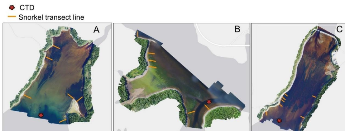
Figure S2.1. Schematic of snorkel transect (orange line) and turbidity sensor (red star) locations for A) North Harbour, B) Swift Current, and C) Baie de l'Eau. Light canvas grey base map was taken from Esri (2018) and projected from WGS 1984 to NAD1983 MTM zone 1 using ArcMap (v.10.7).
