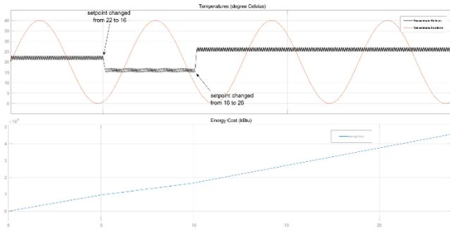
Fig. 9. Indoor temperature and energy cost, when outside temperature is theoretical.
