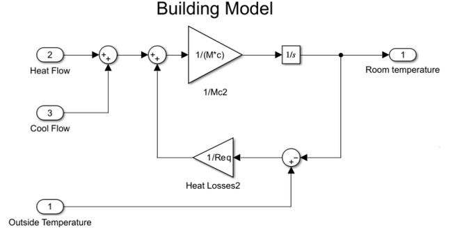
Fig. 7. Building Simulink model.
