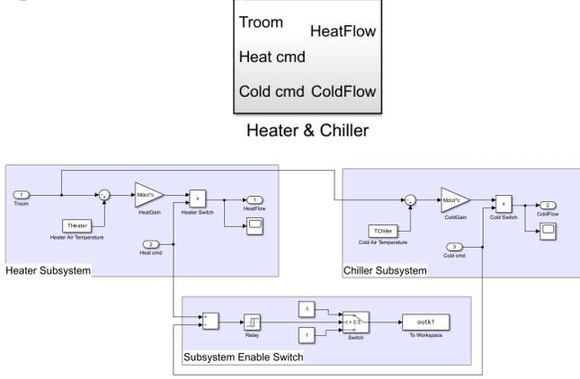
Fig. 6. Heater and Chiller Simulink model.
