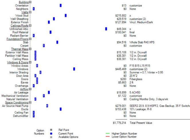
Fig. 3. Overview of BEopt designed inputs.
