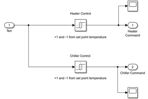
Fig. 5. Thermostat/Controller Simulink model.
