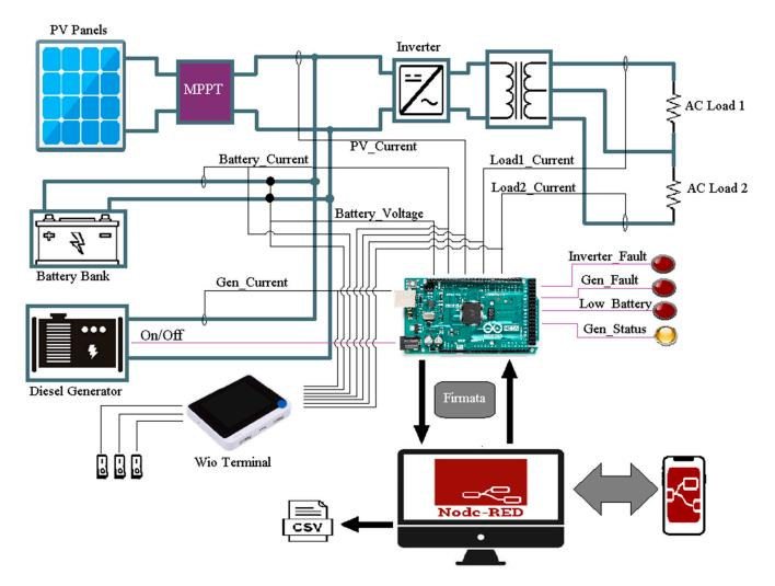
Figure 1. Designed SCADA system for a hybrid renewable power system.
