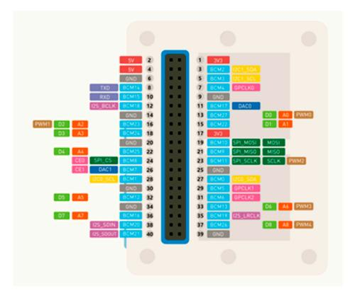
Figure 7. Wio terminal RPI pinout schematic.
