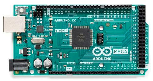
Figure 4. Arduino Mega 2560.
