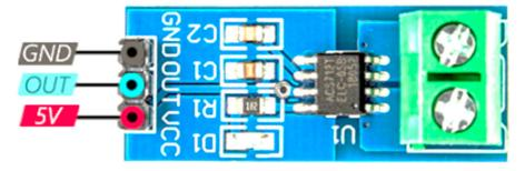
Figure 2. ACS712 current sensor module.
