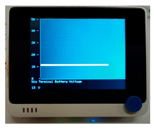
Figure 14. Wio terminal battery voltage display (Mode 1).
