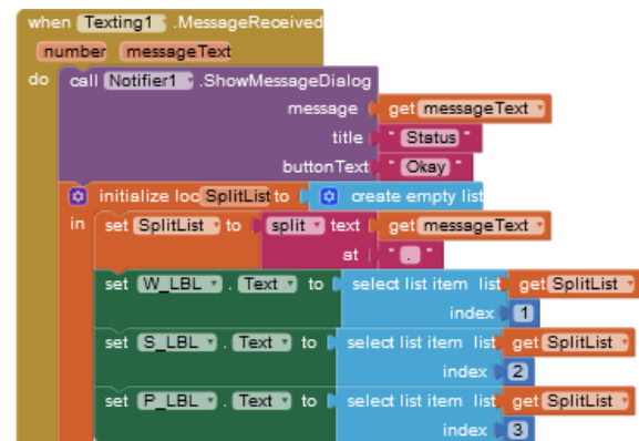
Fig. 6. A section of MIT App Inventor design block when text is received from Arduino and processed to display on app dashboard.
