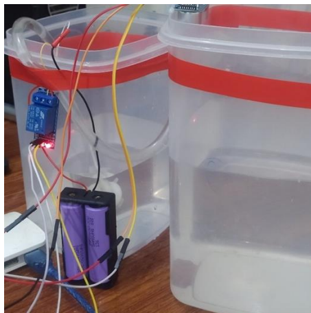
Fig. 3. Two water tanks. The left one represents an underground water storage, while right one represents the outer water storage tank. The underground water tank is installed with a DC water pump that is controlled by Arduino using SPDT relay; and powered by a battery pack of two 18650 Li-ion battery cells. The outer tank is fitted with an ultrasonic sensor.
