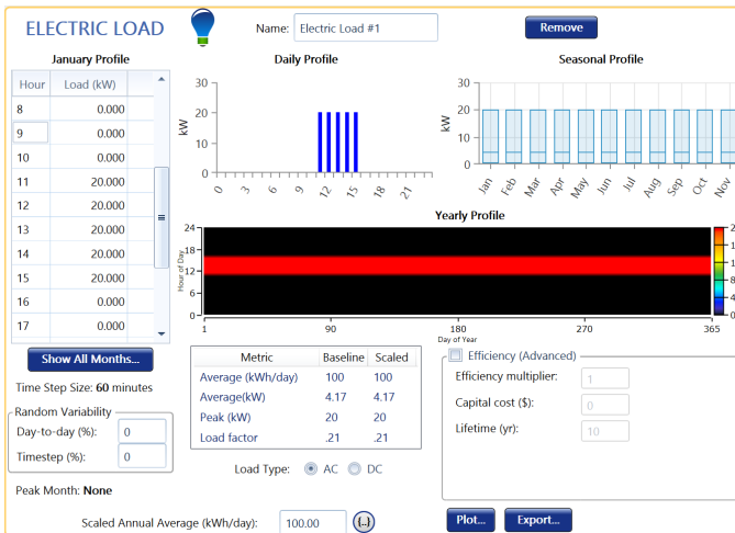
Fig. 8. Load profile when the system runs for 5 hours/day.
