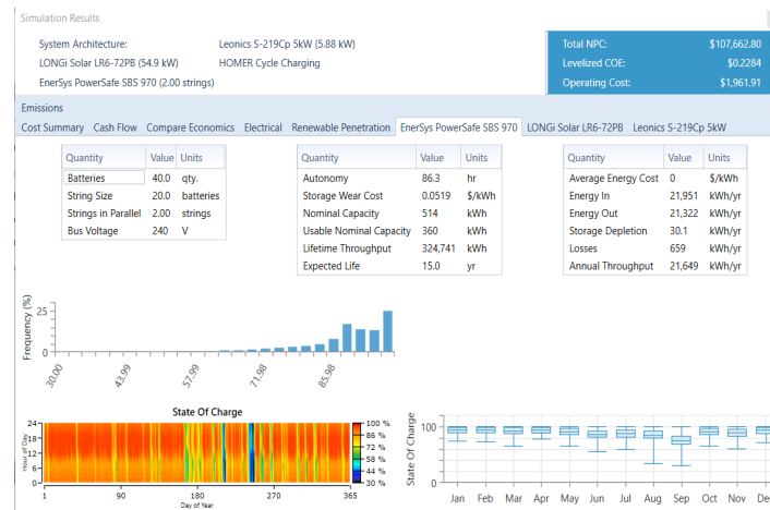
Fig. 16. The battery performance details for the non-stop running time.
