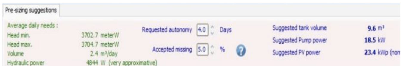
Fig. 7. The pre-sizing suggestion done by PVsyst for a non-stop running time.
