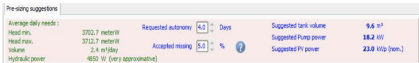
Fig. 6. The pre-sizing suggestion done by Pvsyst for 5 hours running time.
