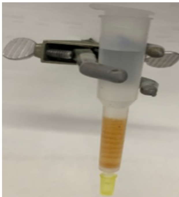
Figure 2.6. A photograph of a 1.66 mL (1 g) bed volume mixed-bed ion exchange chromatography column.
