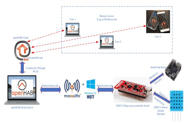
Fig. 13. The communication mechanism.
