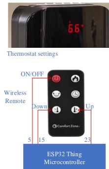
Fig. 8. The connection diagram of remote and ESP32 Thing for thermostat settings.
