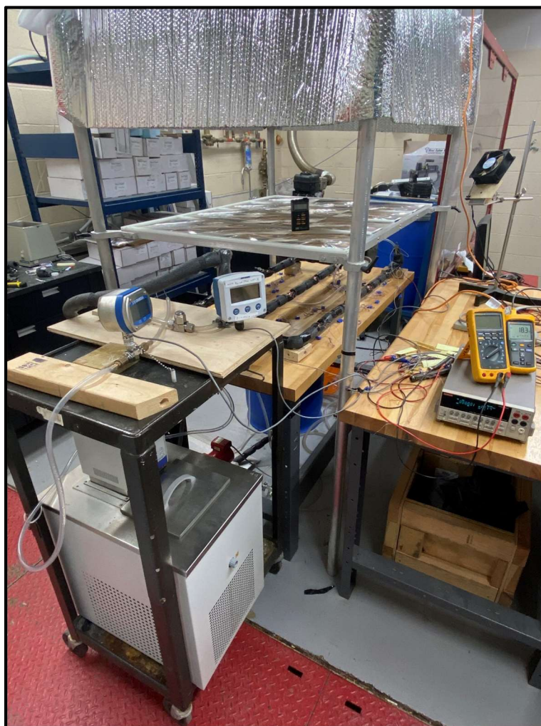
Fig. 3.2: A photo of the test facility with the solar simulator and measuring devices
