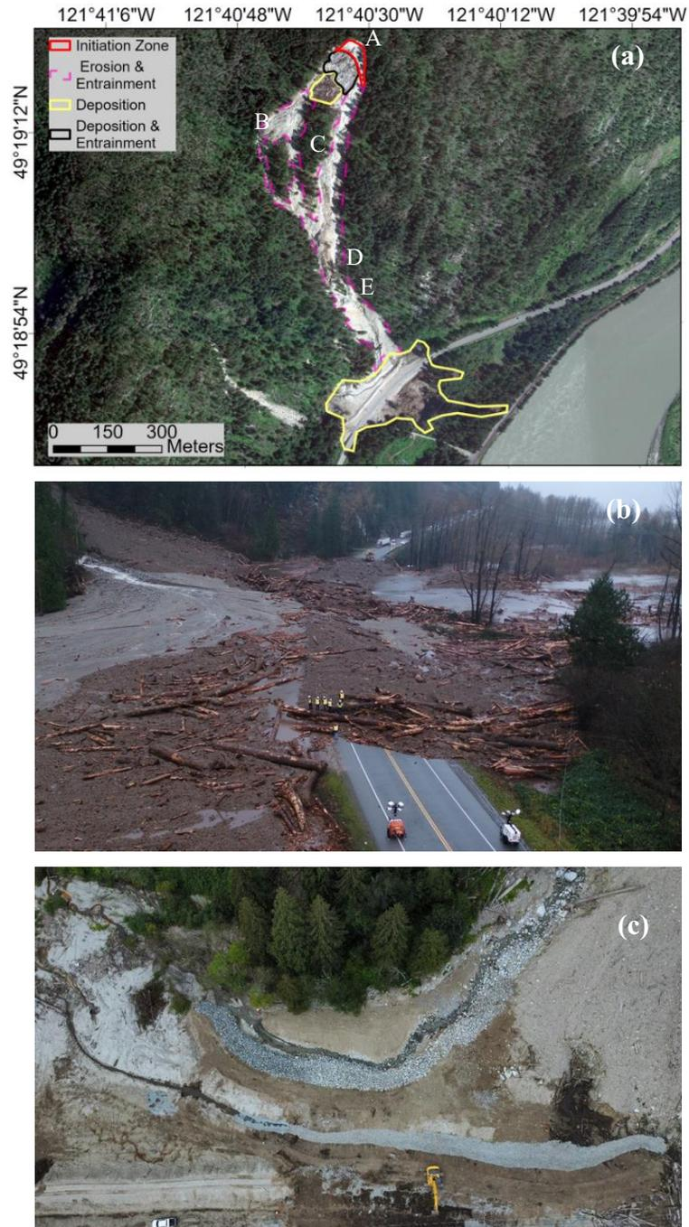
**Fig. 3.1.** Debris flow at Highway 7 between Hope to Agassiz, BC, Canada (Site 1): (a) entire view, (b) view along the highway, (c) view at the toe; Source: Google Earth and BC Ministry of
