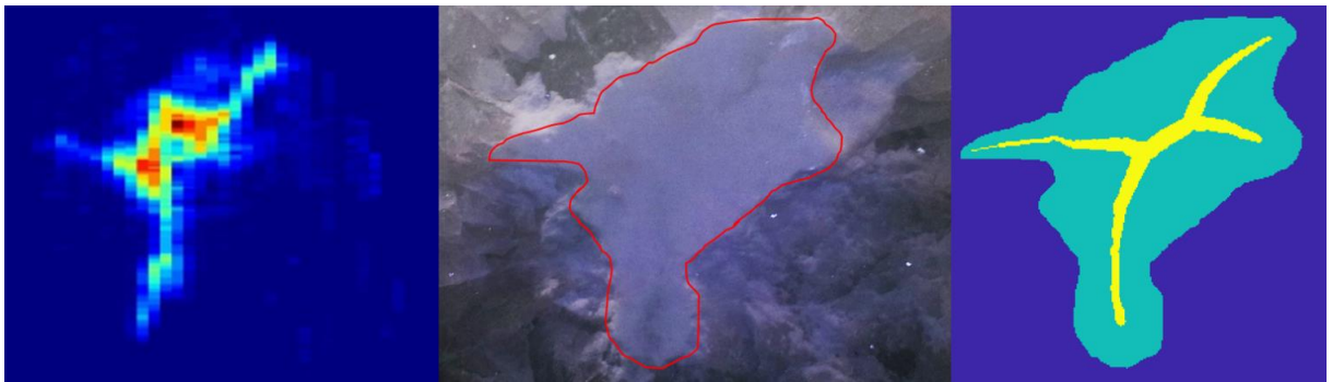
Figure 5-24 – Generated HPZ distribution for Feb25_2016 (Gagnon et al., 2020) test face (centre) using the topological skeleton method (right). It is compared to the pressure map (left). The pressure map is not on the same scale.
