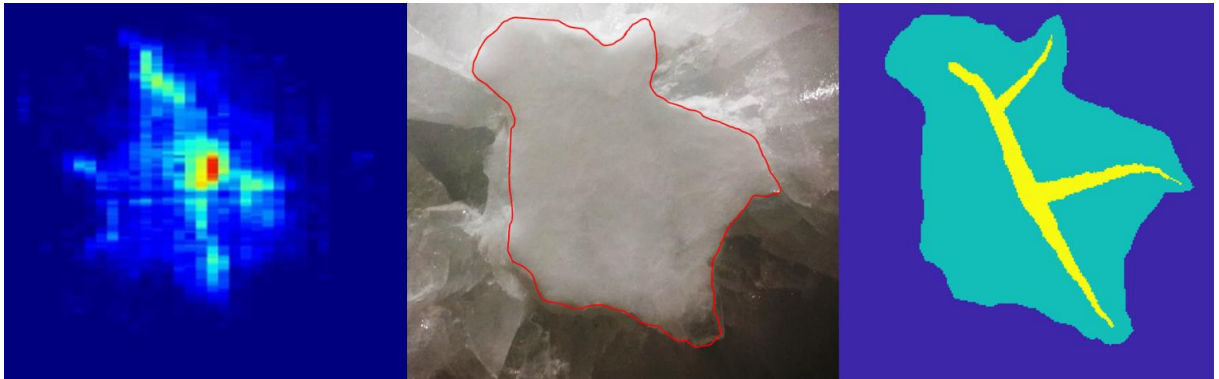
Figure 5-23 – Generated HPZ distribution for Dec10_2015 (Gagnon et al., 2020) test face (centre) using the topological skeleton method (right). It is compared to the pressure map (left). The pressure map is not on the same scale.
