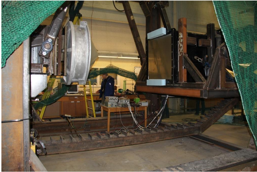
Figure 2-2. Photograph showing a partial view of the double-pendulum impact apparatus with the ice holder pendulum (left) and Impact Module pendulum (right) in the raised position for a test. The ‘toothed’ rail structure directly below the pendulums is the catch mechanism as shown in Fig. 1. Protective netting is visible at the sides and in the background of the image. An overhead crane is used for lifting the pendulum masses to the desired elevation for a test.
