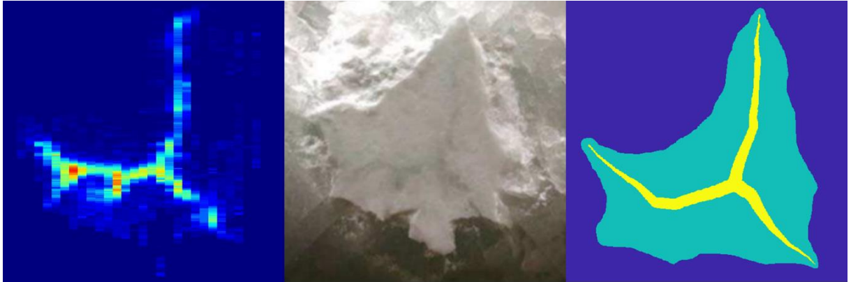
Figure 5-20 – Large pendulum’s ice impact October16_2014 test face (centre) compared with experimental pressure distribution data, and the HPZ distribution predicted by the topological skeleton methodology (left). Images are not on the same scale.
