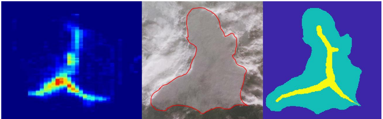
Figure 5-22 – Generated HPZ distribution for Jan20_2015 (Gagnon et al., 2020) test face (centre) using the topological skeleton method (right). It is compared to the pressure map (left). The pressure map is not on the same scale.
