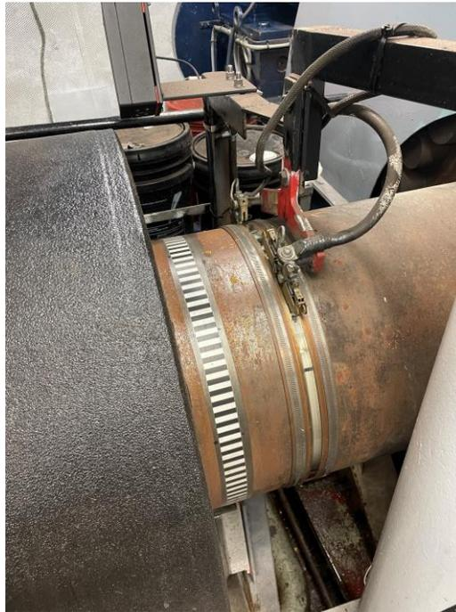
*Figure 3 - TT Sense ® mounted on CCGS Henry Larsen port shaft.*
