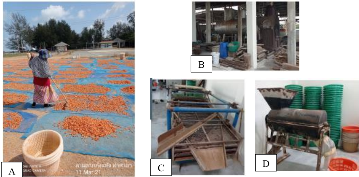
Figure 4.3. Dried shrimp processing and equipment. A. Shrimp drying in a shared area in Tha Sala, Nakhon Si Thammarat; B. Shrimp boiler; C. Sorting machine; D. Shell remover machine. (Photo credit: DFM Thailand Team, 2021)
