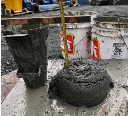
Figure 4-6: Slump test for the backfilling mixtures using SL aggregates
