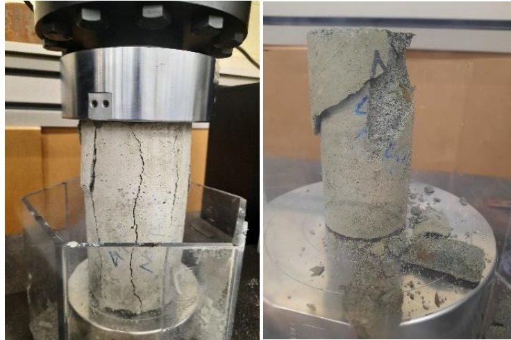
Figure 3-7: Cylindrical Samples of CPB for UCS Testing in the Instron Loading Frame
