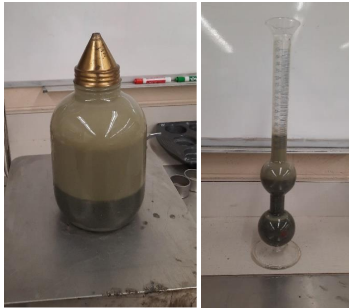
Figure 3-2: Specific Gravity Determination using Pycnometer and Le Chatelier Flask
