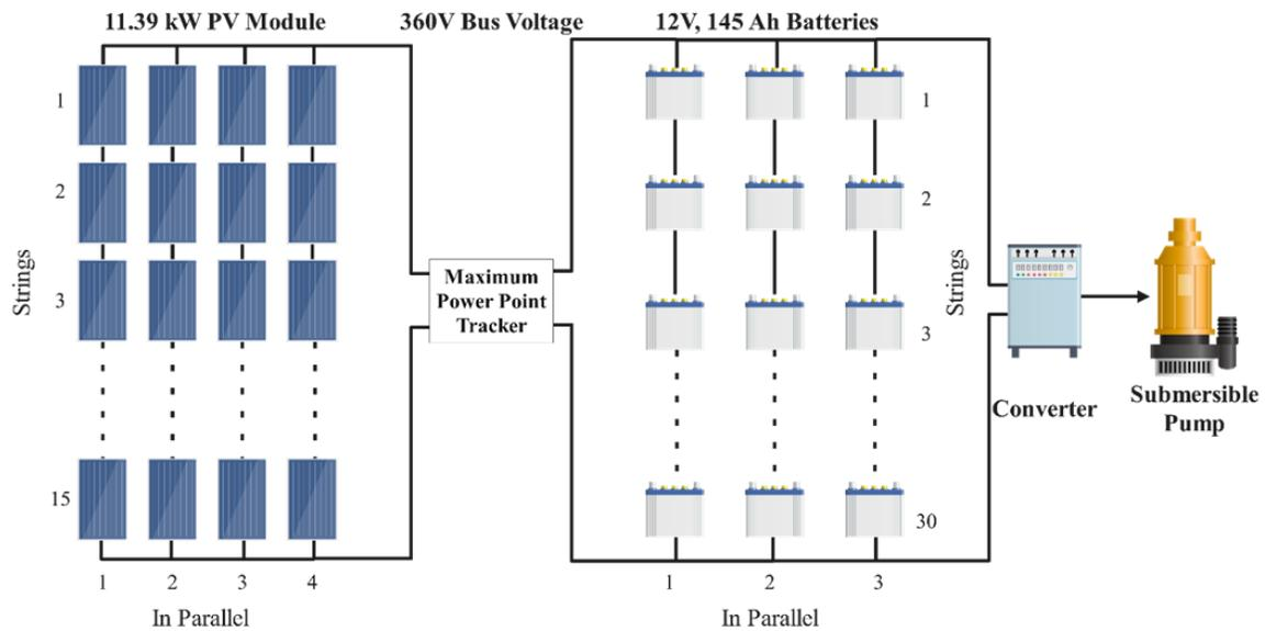
Figure 2.6 Configuration of proposed system
