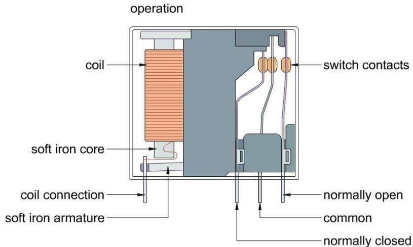
Figure 3.6 A general structure of SPDT Relay
