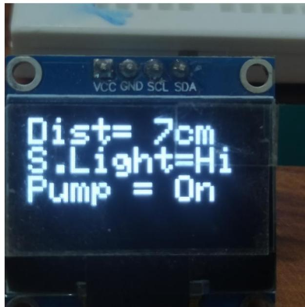
Figure 3.9 Status displayed on OLED of PV water pumping system.
