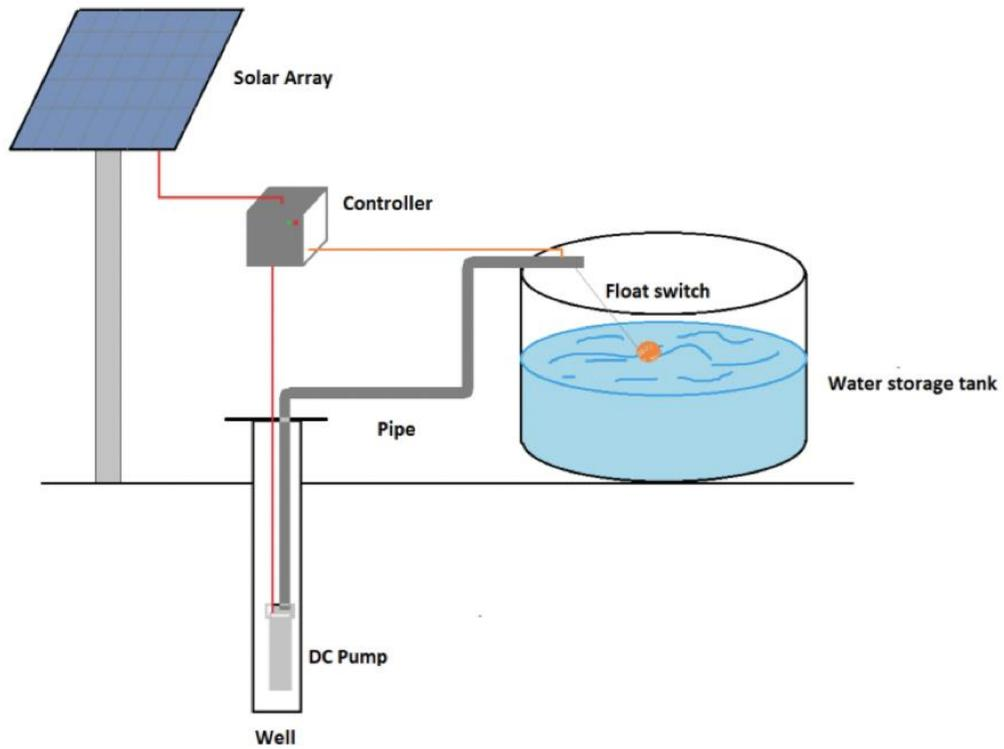
Figure 1.4 Constituents of solar powered water pumping systems.
