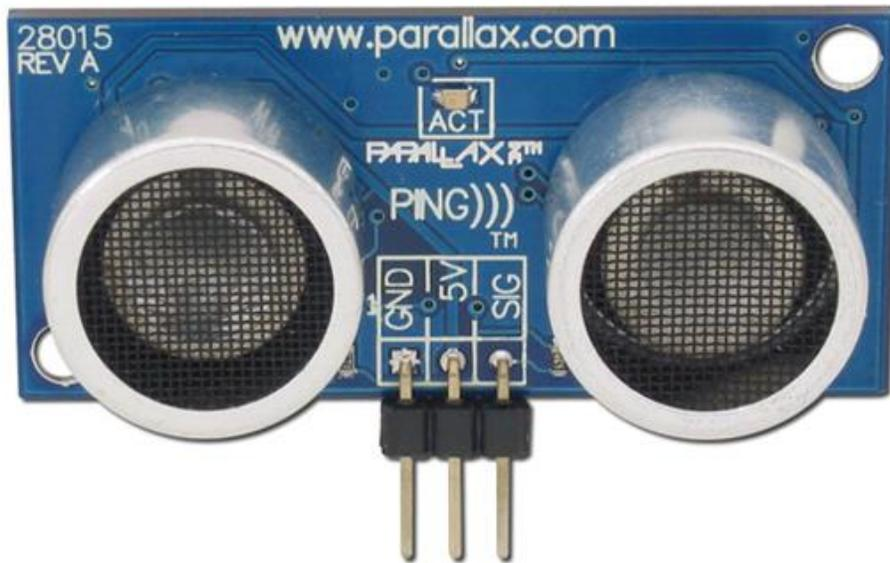
Figure 3.3 An Ultrasonic Sensor for displacement measurement
