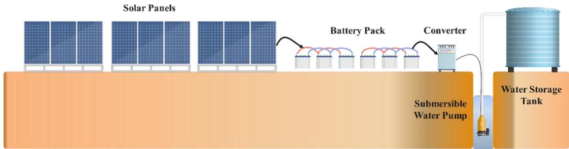
Figure 2.5 Schematic of deep well system
