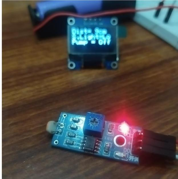
Figure 3.12 LDR module with OLED in background
