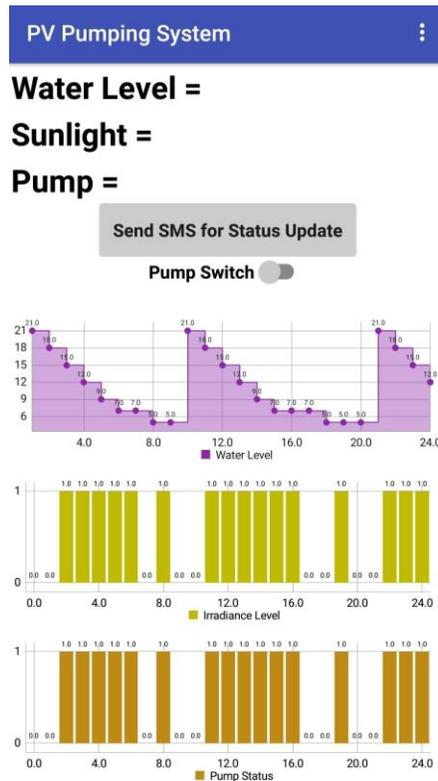
Figure 4.8 User Application designed in MIT App Inventor
