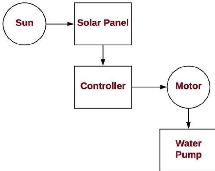
Figure 1.3 Solar Water Pump Block Diagram
