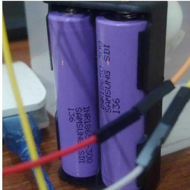
Figure 3.10 Two 18650 Li-ion Battery Cells to power up the DC pump
