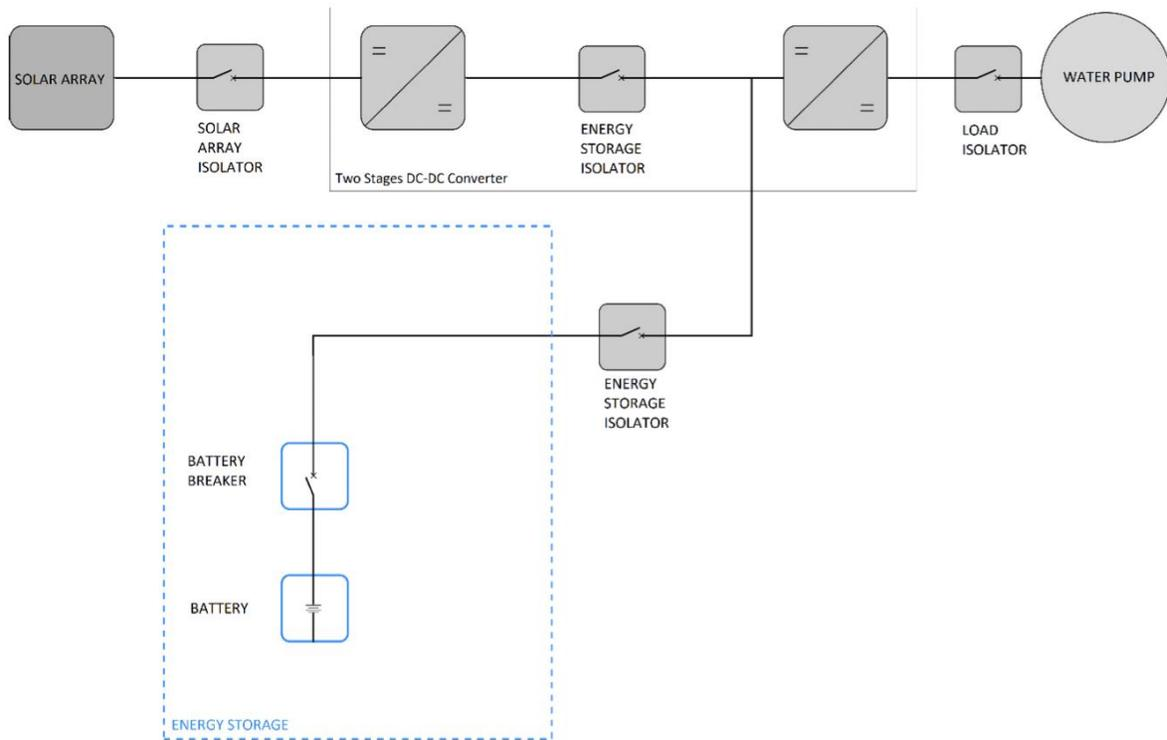
Figure 1.2 Isolated PV solar water pumping system
