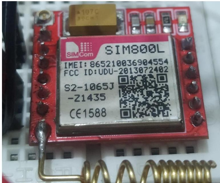
Figure 3.5 GSM Moudle SIM 800L
