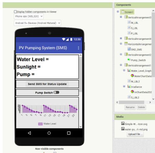
Figure 4.6 An android mobile app is designed using MIT App Inventor.
