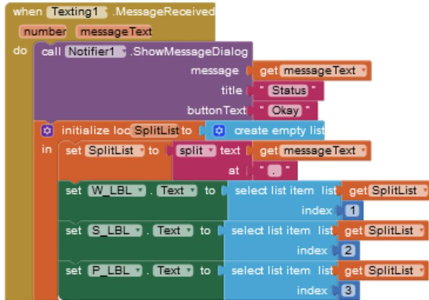
Figure 4.5 A section of MIT App Inventor design block when text is received from Arduino and processed to display on app dashboard.
