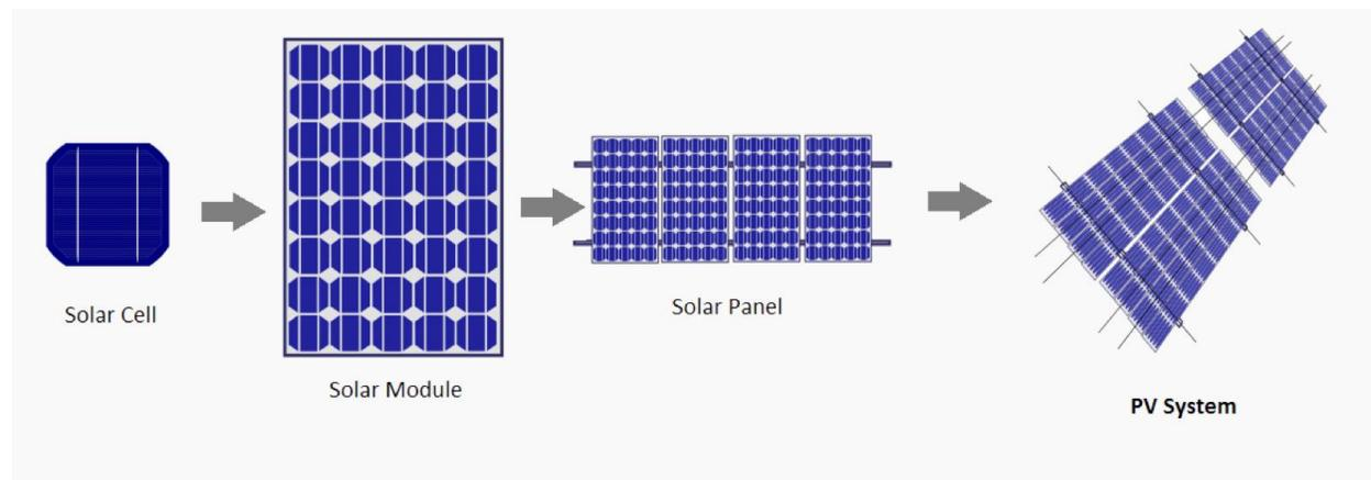
Figure 1.1 PV system constructed from PV module
