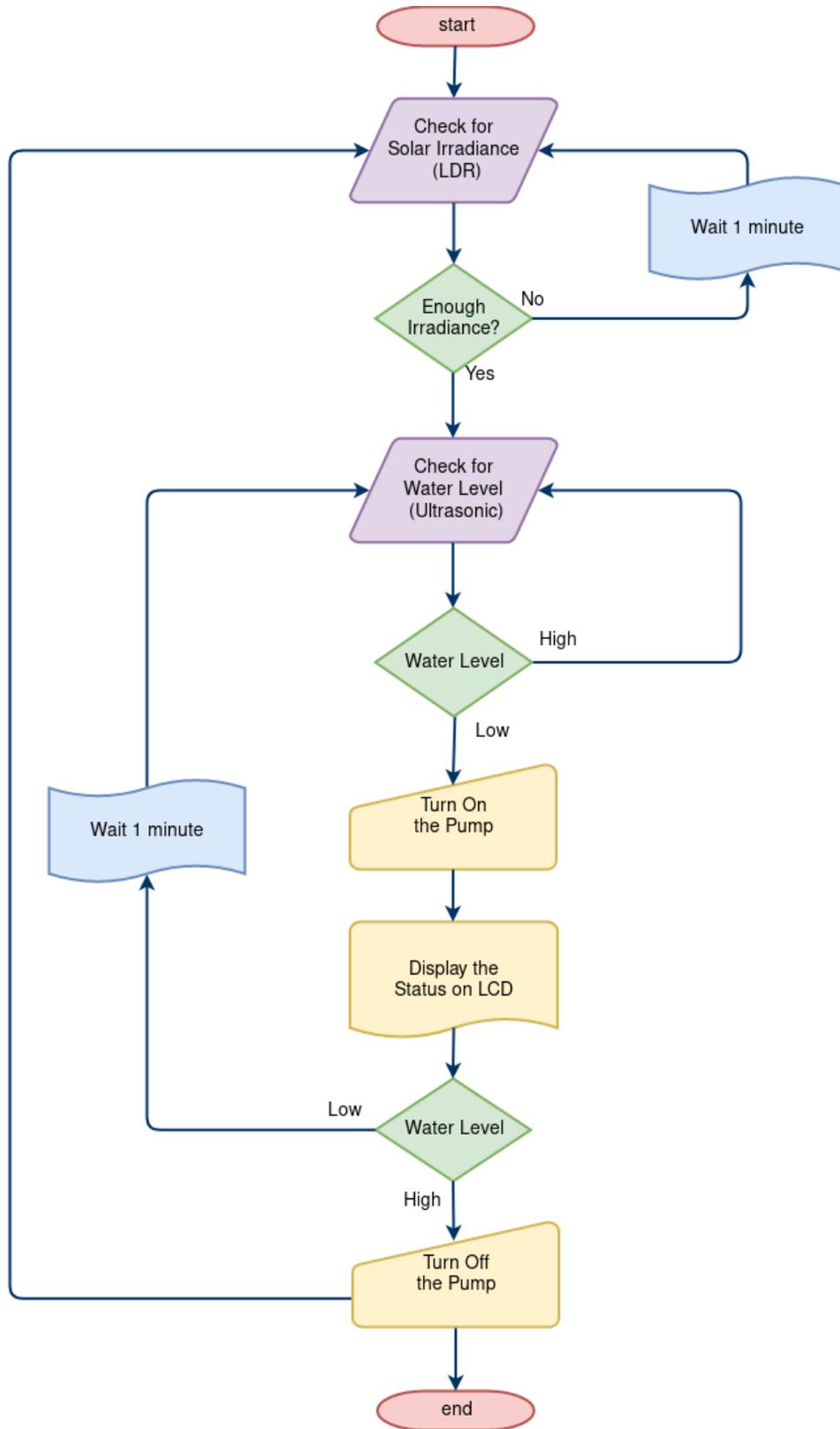
Figure 3.7 Flowchart of the control strategy of PV water pumping system
