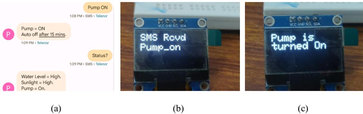
Figure 3.14 User prompt regarding turning the pump on
