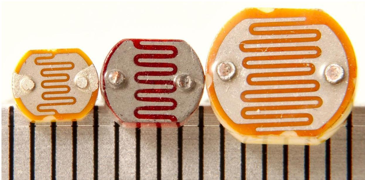
Figure 3.4 A set of photoresistors
