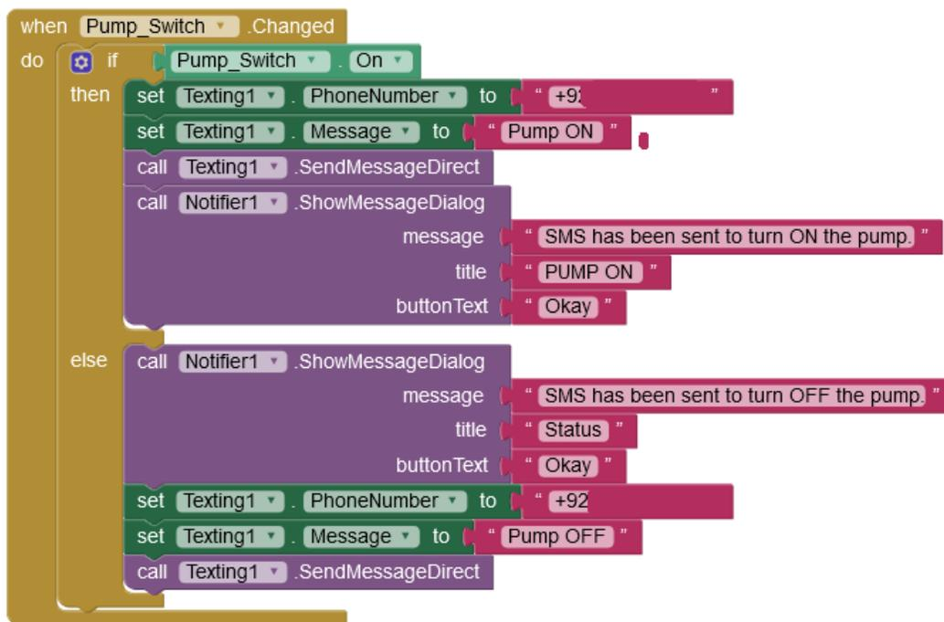
Figure 4.4 MIT App Inventor design block to turn on and turn off the pump on user discretion.
