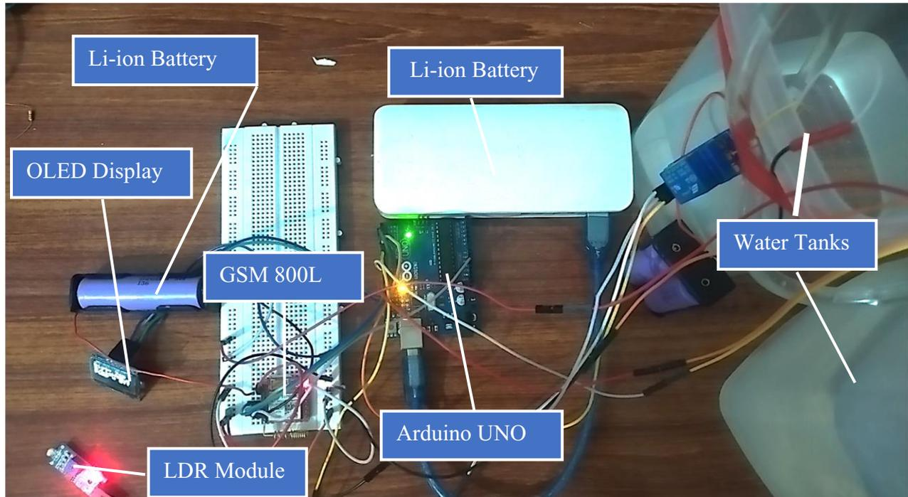
Figure 4.1 Test Hardware Setup of the proposed system
