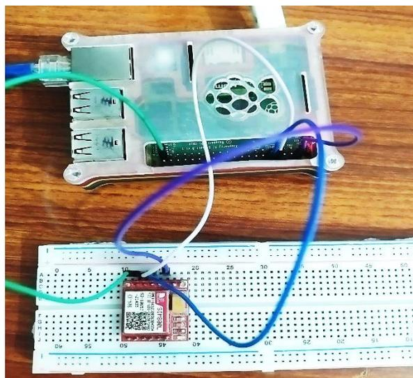
Figure 4.2 GSM module connected with Raspberry Pi 2.
