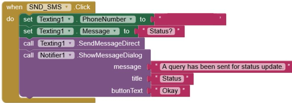
Figure 4.3 A design block in MIT App Inventor when a query is generated from user app.
