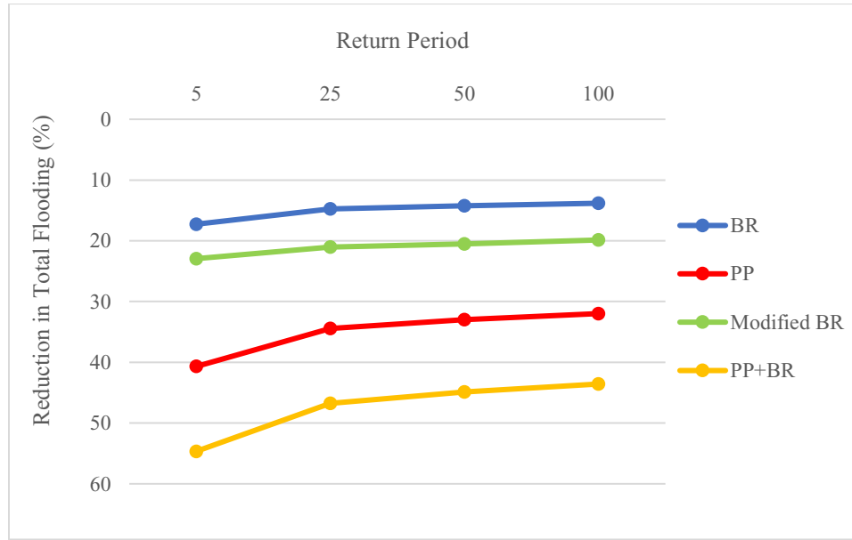
Figure 27. Reduction of total flooding (%) by different LID options: Permeable Pavement (PP), Bioretention (BR), and the combinations (BR+PP, Modified BR).
