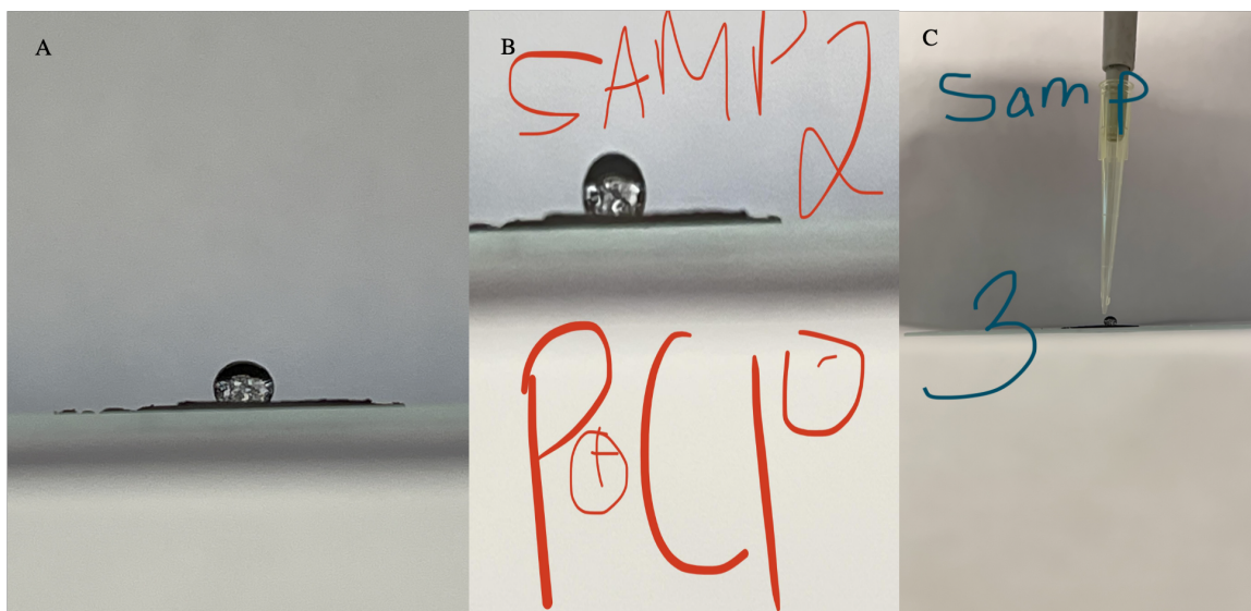
Figure SI 2.2 The contact surface angle measurements of exfoliated indirect synthesis of (\text{C}_8\text{H}_{17})_3\text{P}^+\text{Cl}^- biochar.
