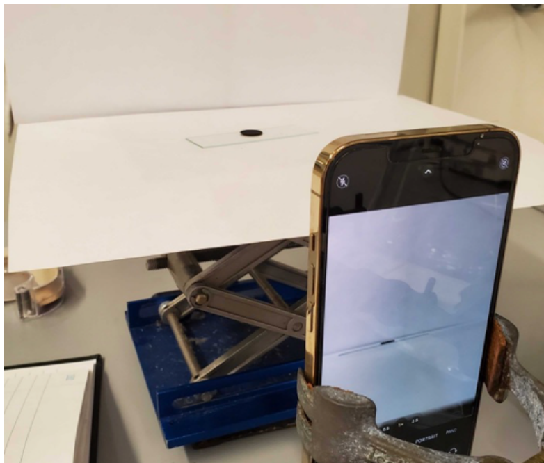
Figure SI 2.1 Surface contact angle experimental setup
