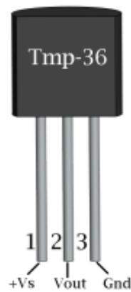
Figure 3:8: TMP36, Temperature Sensor.
