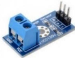
Figure 3:4: Voltage Sensor image
