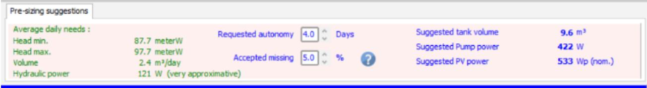
Figure 2:14: Pre-sizing parameter, simulation parameters and results
