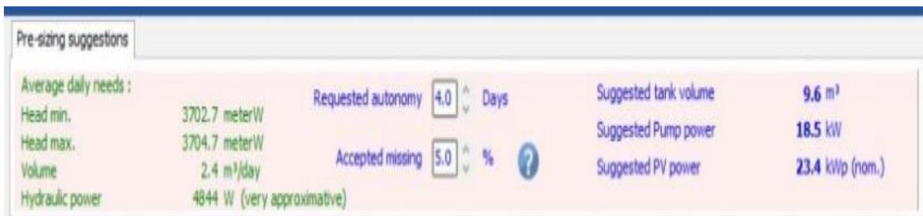
Figure 2:4: PVsyst system sizing Suggestion
