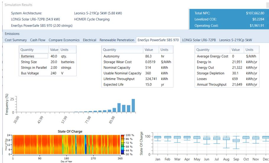
Figure 2:13: Battery performance details for 24 hours running time
