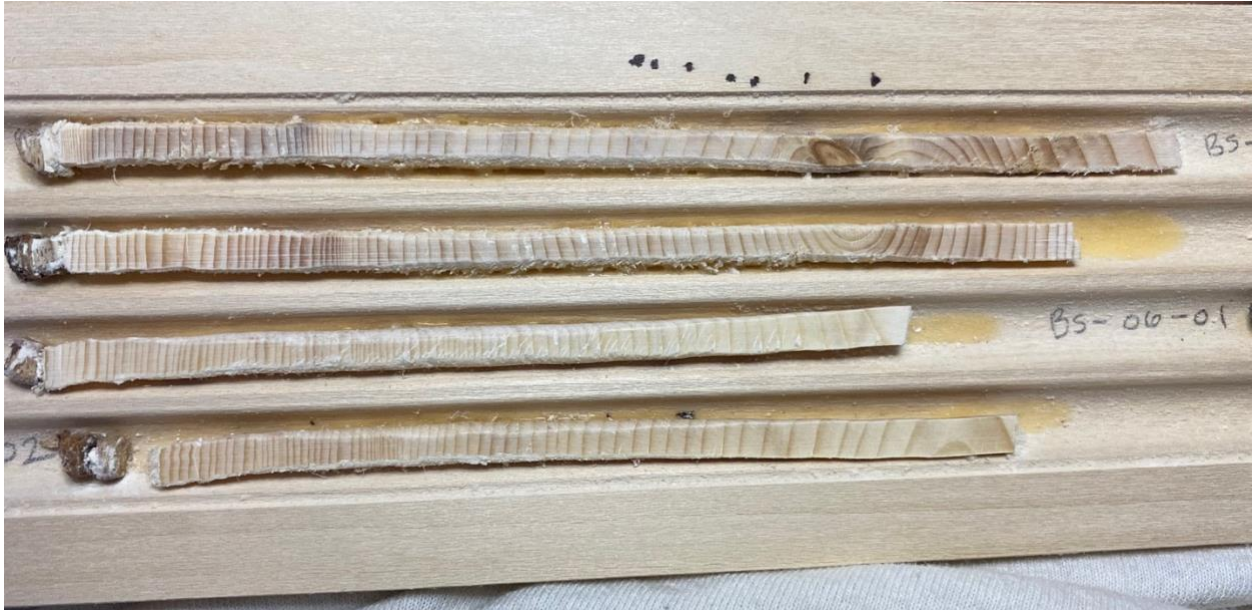
Figure 2.5 Mounted and sanded black spruce tree cores. Cores were sanded using a belt sander with progressively finer grit from 80, 120, 180, 220, 400, and 600 grit. The latewood (i.e., dark rings) was counted to estimate age.
