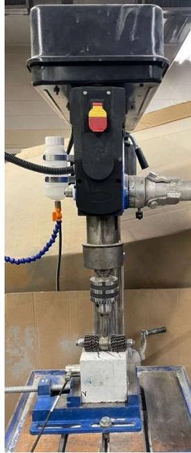
**Fig. 2- 2** Rotating cutter abrasion test setup.
