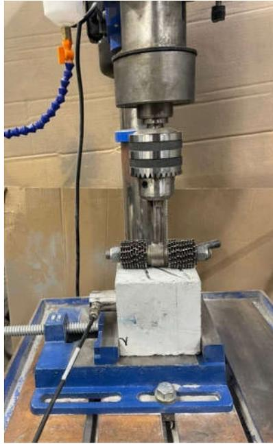
**Fig. 4- 1** AE and rotating cutter abrasion test setup.
