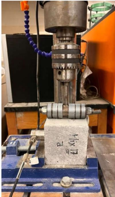
**Fig. 4- 2** Verification abrasion test setup using a smooth roller.
