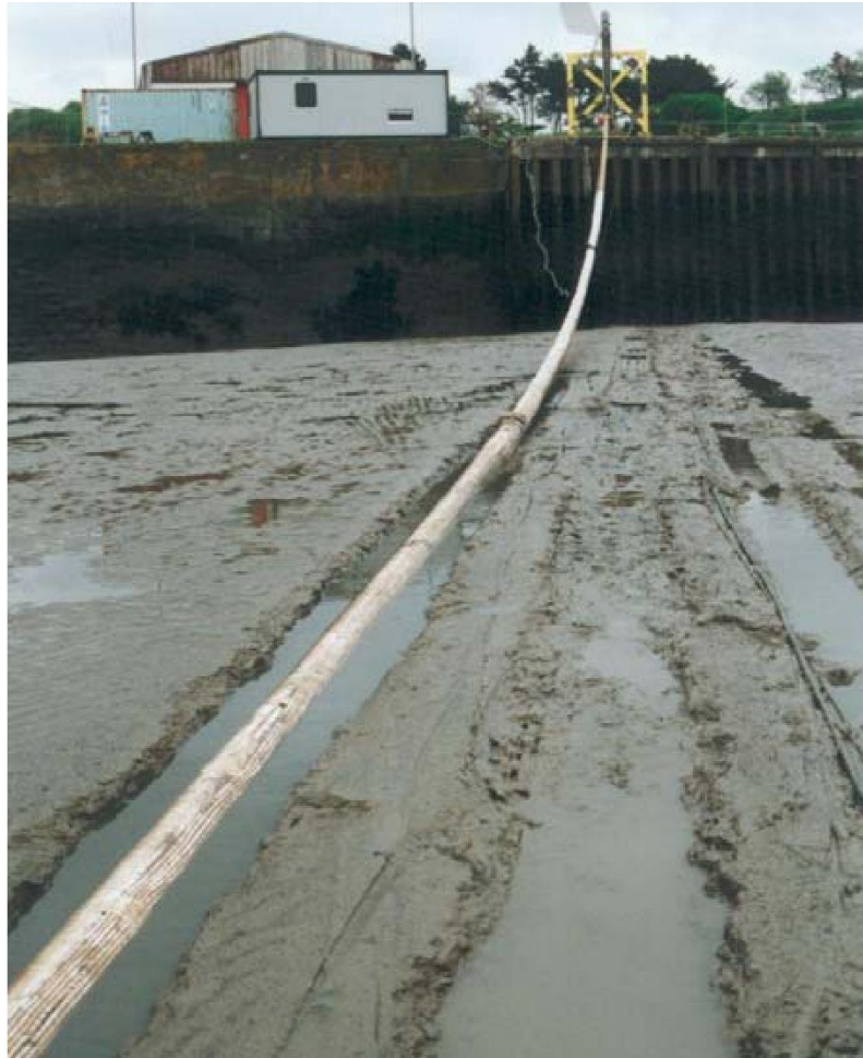
Figure 2-3. SCR-seabed-seawater interaction observed in SCR full scale test, Watchet Harbor, UK (Bridge & Willis, 2002)
