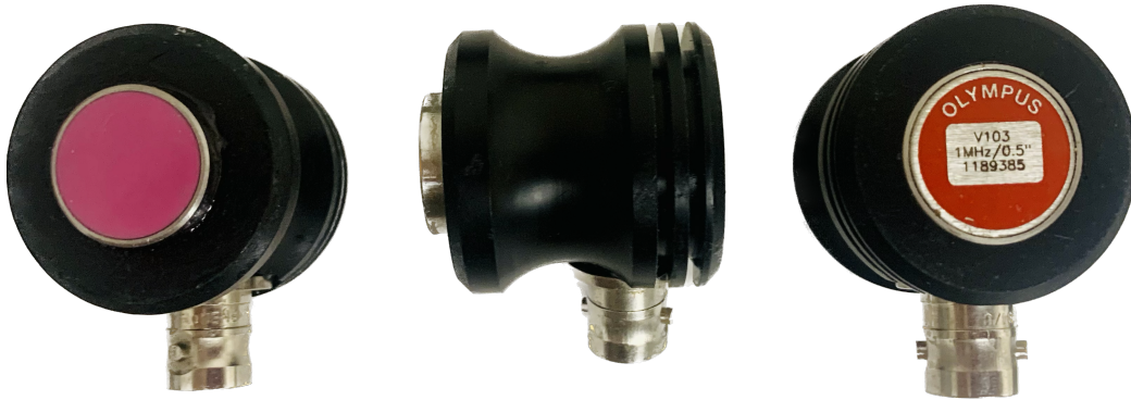
Figure 2.12: Olympus ultrasonic contact transducers. Our P-wave and S-wave transducers are identical in appearance but distinguishable by serial numbers.
