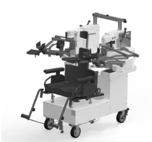
Figure 1.2 Kinarm Exoskeleton (Left side), Kinarm Endpoint (Right side). The images above depict two types of Kinarm robot devices. On the left is the exoskeleton type, while on the right side is the endpoint type. © Copyright BKIN Technologies 2023. All Rights Reserved (Received Permission to use).
