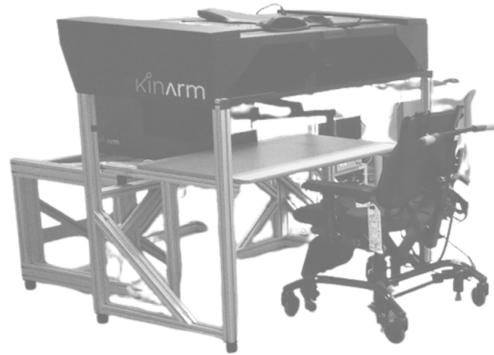
Figure 1.2 Kinarm Exoskeleton (Left side), Kinarm Endpoint (Right side). The images above depict two types of Kinarm robot devices. On the left is the exoskeleton type, while on the right side is the endpoint type. © Copyright BKIN Technologies 2023. All Rights Reserved (Received Permission to use).
