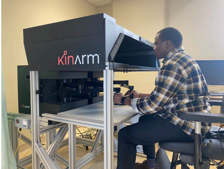
Figure 2.5b Example of subject positioning using adjustable Kinarm electronic chair while performing Object Hit and Avoid Tasks. (Original Image by MB).
