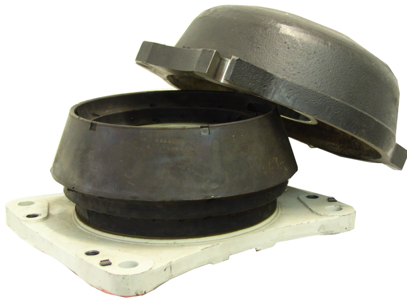
Figure 2.3: Components of the conical resilient mount under test
