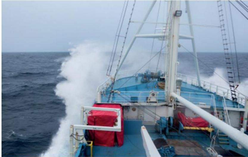
Figure 1. 4: How icing occurs through sea spraying (Kulyakhtin & Tsarau, 2014)
