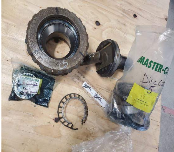
Figure 5-1. Disassembled disc cutter parts.
