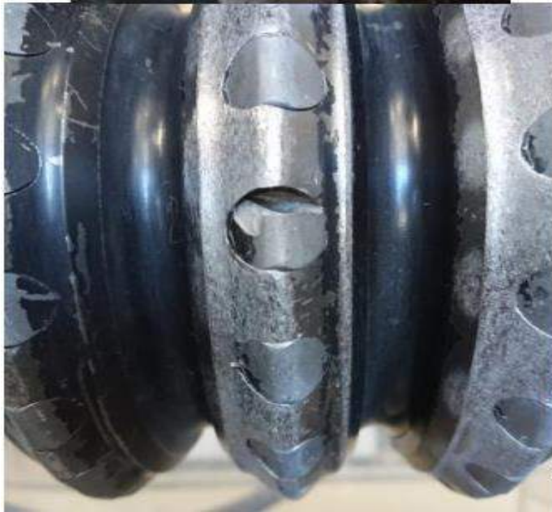
Figure 4-9. Diagram of a chipped insert.
