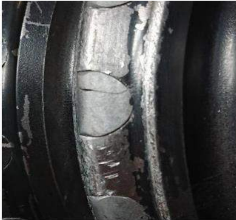
Figure 4-8. Diagram of a fractured insert.
