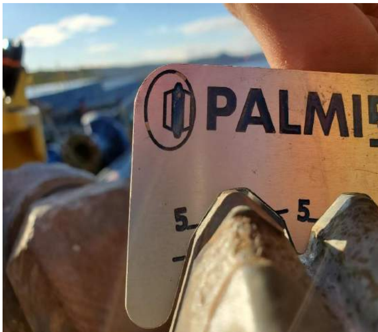
Figure 3-2. Image of Wear Gage used on the field. (Tytler et. al., 2022)
