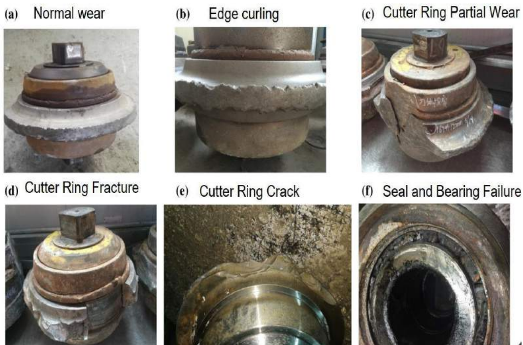
Figure 2-1. Different types of disc cutter wear
