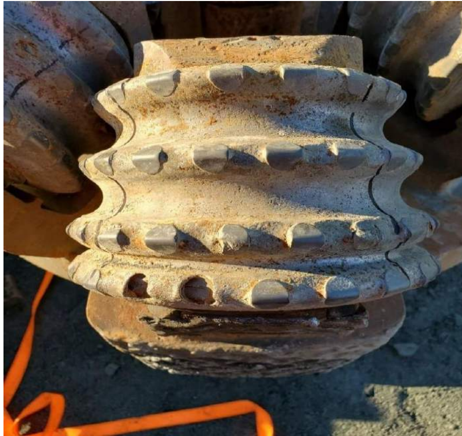
Figure 3-1. Damaged multi-edge disc cutters (Novamera Inc., 2022).
