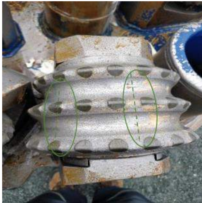
Figure 4-6. Diagram showing extended lines across the top of the cutter.
