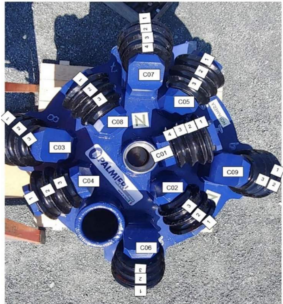
Figure 4-4. Diagram of a fully labeled cutter head.
