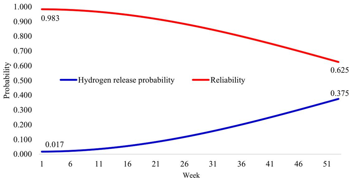
Figure 3. 5 Dynamic modeling of hydrogen release probability and the system reliability using DBN
