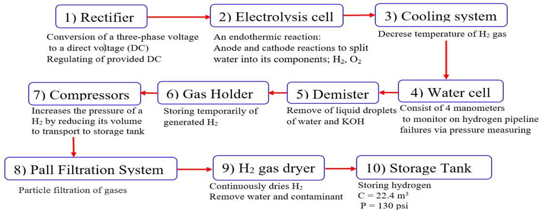
Figure 3. 2 A block diagram of hydrogen generation plant by alkaline water electrolysis.
