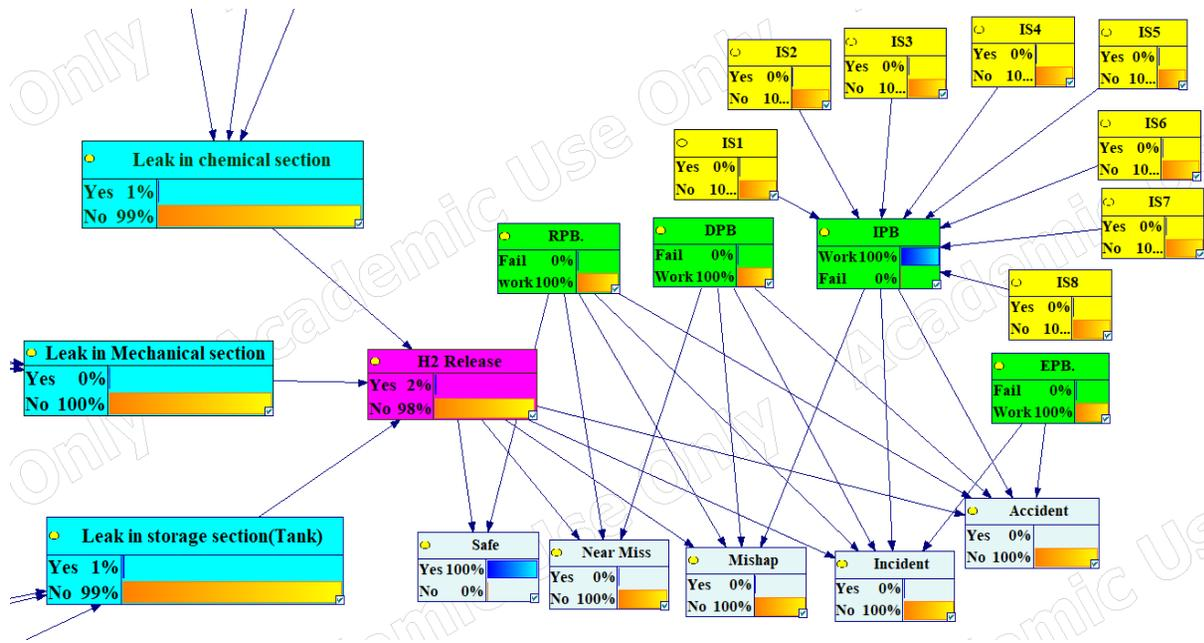
Figure 3. 4 Causality modeling of the cause-effect model of the hydrogen release accident scenario
