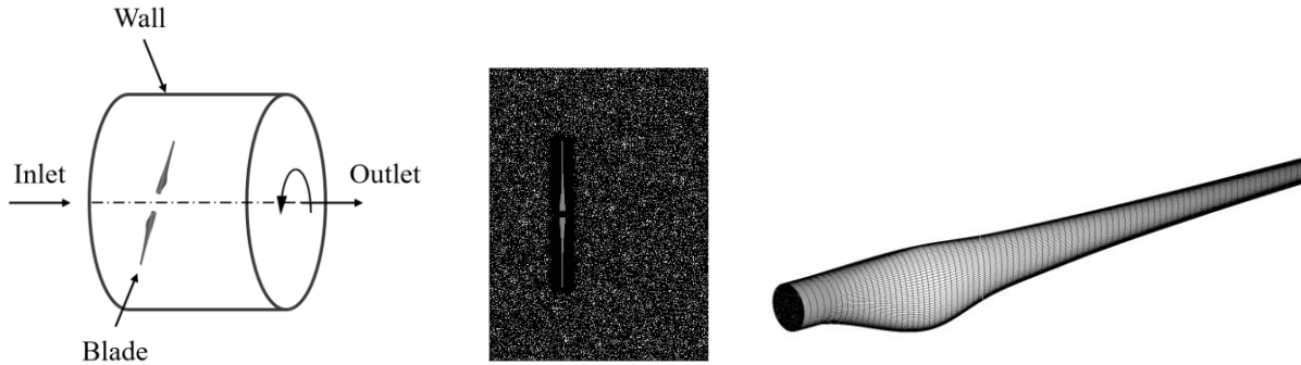
Figure 5.5. Discretization of the CFD grid boundary conditions, Grid sectional view and blade grid surface.
