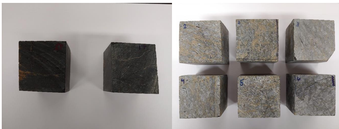
Fig. 4. Tablelands (left) and White Hills (right) rock cubes used for sequestration experiments.
