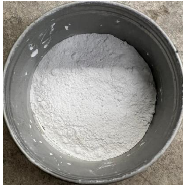
Figure 4.1 Binder Modifier (a) SBS and b) Anti-stripping agent Zycotherm
