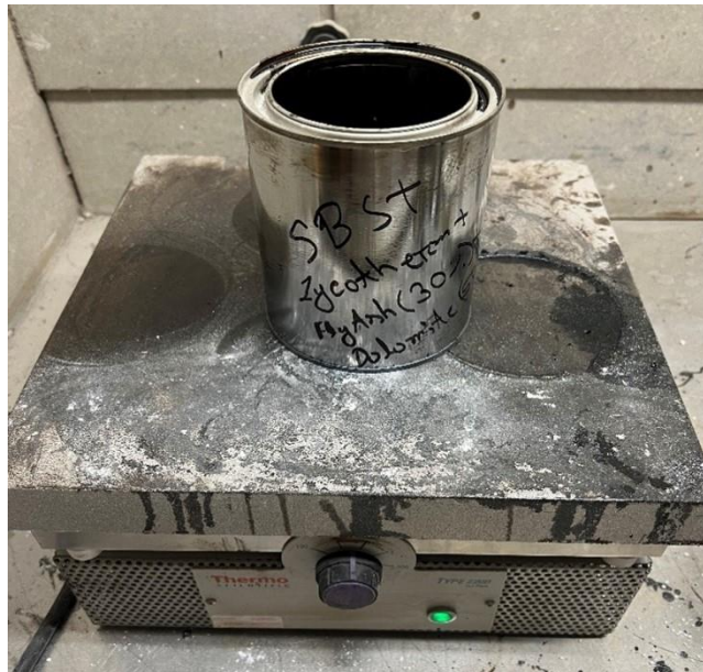
Figure A.2: Pre-heating before mixing
