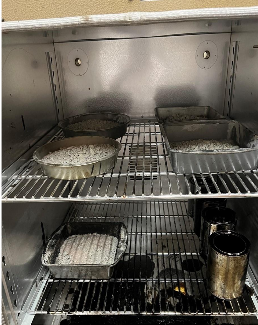
Figure A.8: Pre-heating of aggregates and binder for Marshall test
