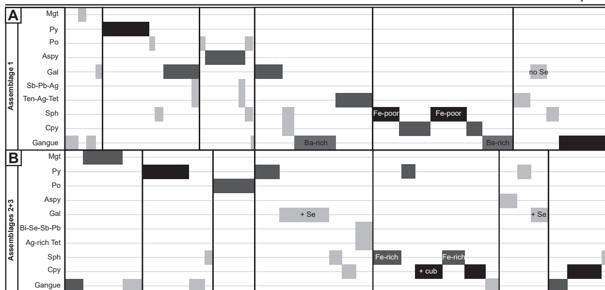
Figure 4.9. Mineralization paragenesis at the ABM deposit. (A) Paragenesis for assemblage 1. (B) Combined paragenesis of assemblages 2 and 3. Black color of bars indicates modal abundances >30 %, dark grey indicates modal abundances between 30-10 %, and light grey indicates modal abundances <10 %.
