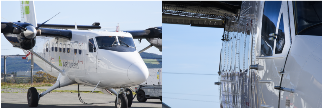
Figure 5.8. Twin otter aircraft used for measurements. Locations of rear-facing inlets for atmospheric air sampling are shown on the right. The AIMMS-30 air data probe can (red) is visible on the left photo.
