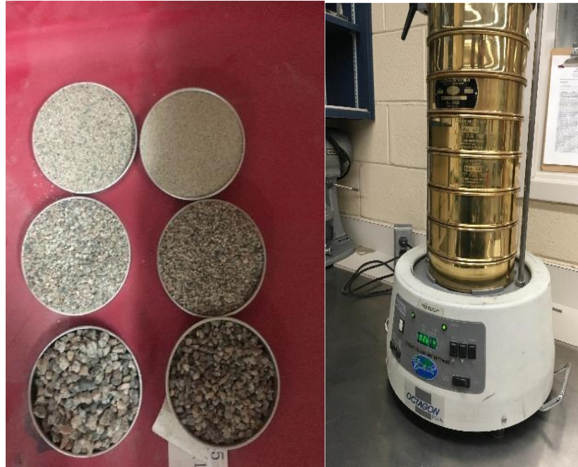
Figure 2. Sieving and Classification of the sand
