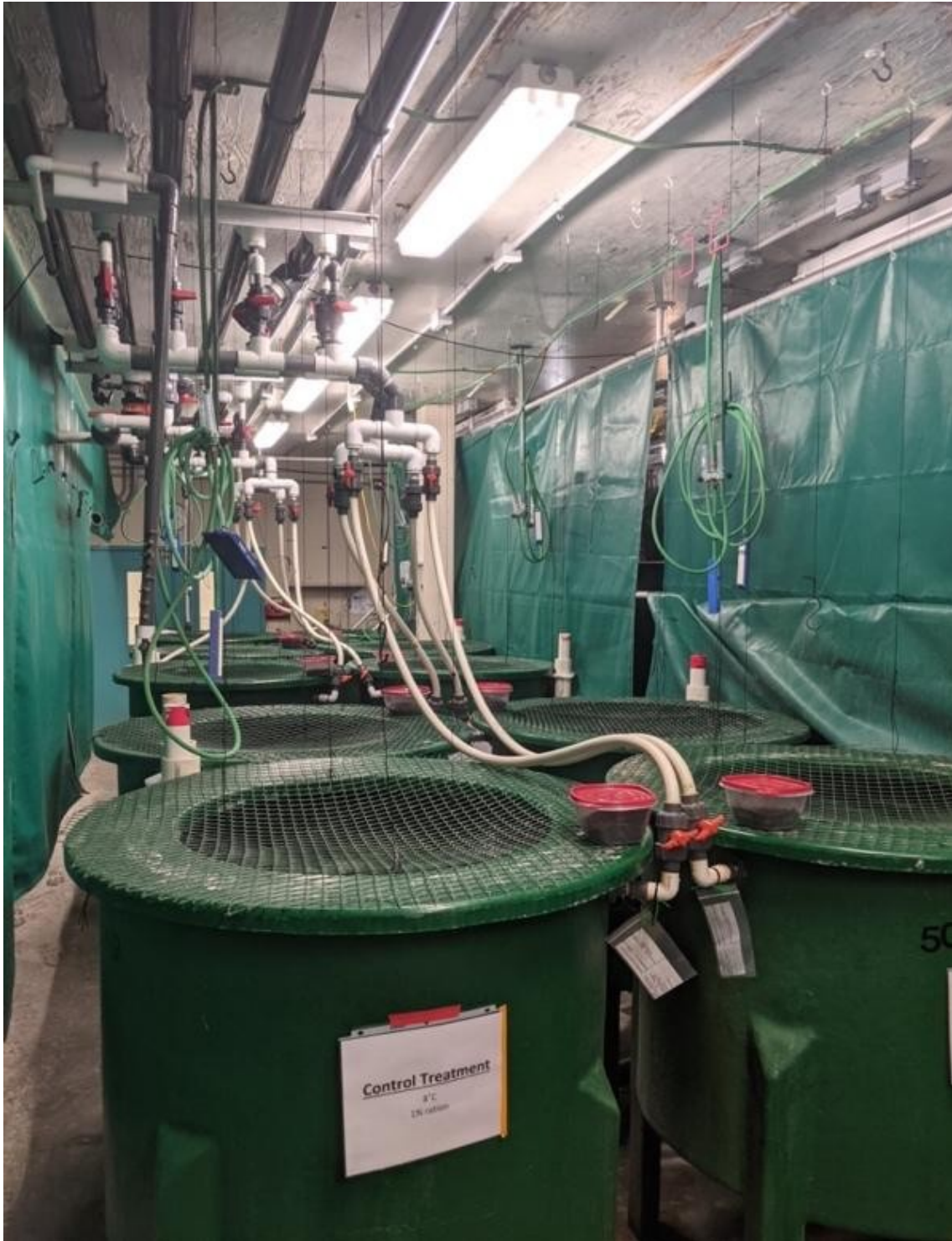
Figure S2. Tanks used in the experiment conducted in Chapter 2. All 8 500 L tanks were connected to 2 flow-through seawater sources (8°C and ambient) so that specific water temperatures could be obtained. Photoperiod was 12h light : 12h dark. Curtains were used on both sides of the tanks to minimize stress disturbance.
