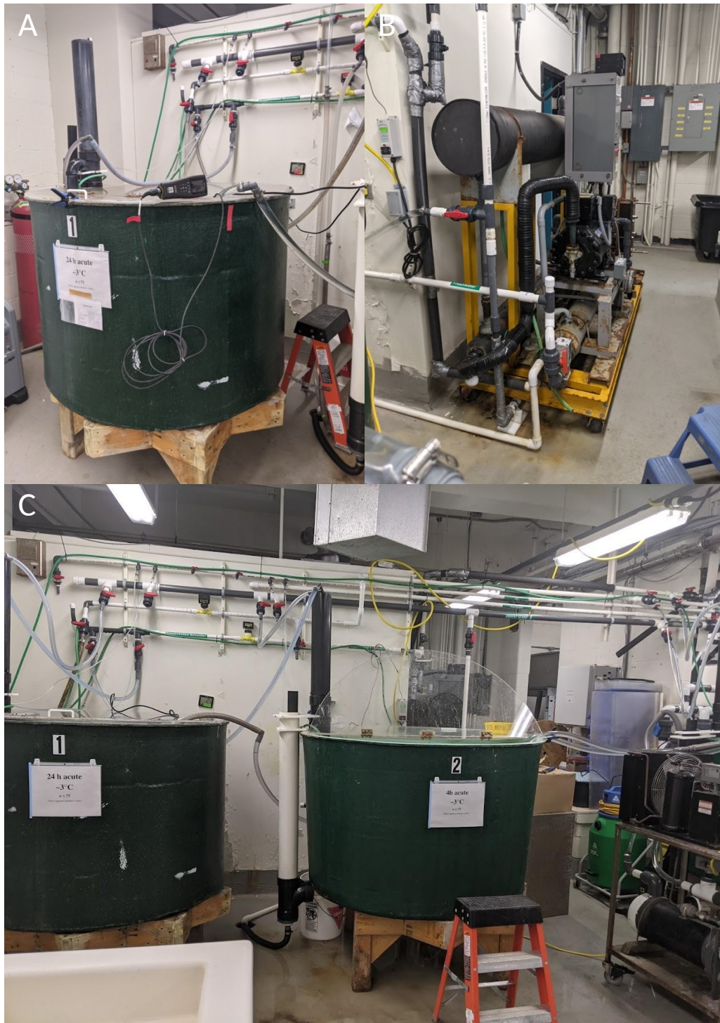
Figure S12. Tank set-up (A, C) for Chapters 3 & 4 including the large capacity glycol chiller (B) used to hold temperatures at 0°C. The fish were held in three 1000 l-tanks (75 and 35 fish per tank for Experiments #2 and #3 respectively). The tanks were in a flow through configuration and supplied with 32 ppt seawater at 7 l min -1 . Each tank was used for a different acclimation group in Experiment #3.
