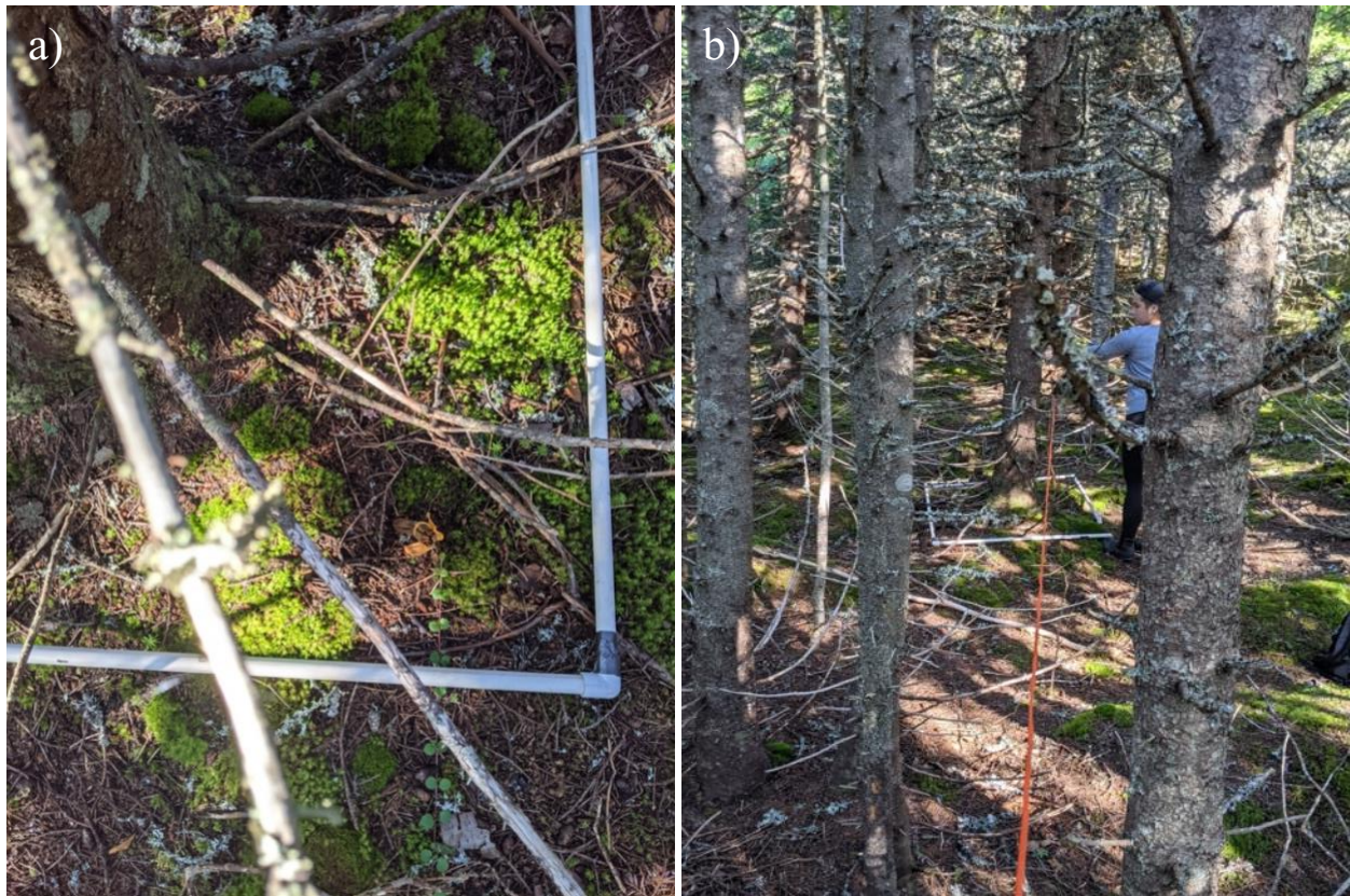
Figure 2.6: Layout of a) small 1m x 1m plot and b) large 5m radius plot. Small plots were established with PVC pipe surrounding a tree that acted as the centre of the plot where the four corners were placed in the four cardinal directions. Large plots were established using a 5m plot cord with a tree representing the centre of the plot.
