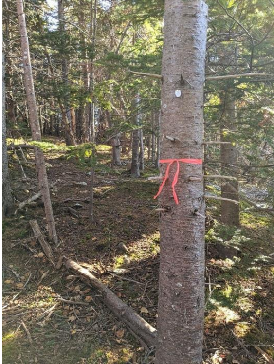
Figure 2.8: iButton Thermochron datalogger attached to the trunk of a tree in a peri-urban site. Datalogger is approximately 1.8m above ground, on the north side of the tree. Photo is taken facing south.
