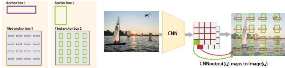
Figure 4-6: How the anchor box works in the faster RCNN object detector
