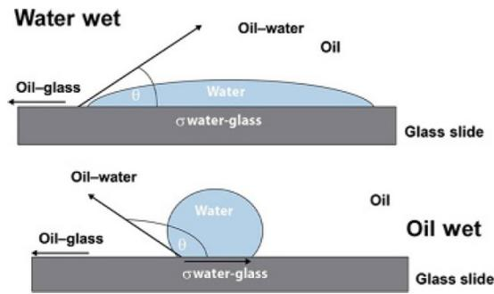
Figure 2-1: Illustration of wettability measurement through contact angle [31]
