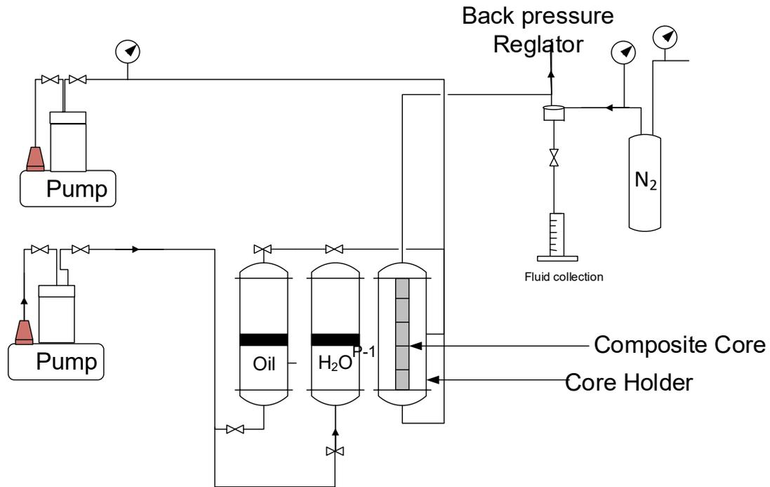
**Figure 5-2: Schematic experimental set-up for coreflooding.**
