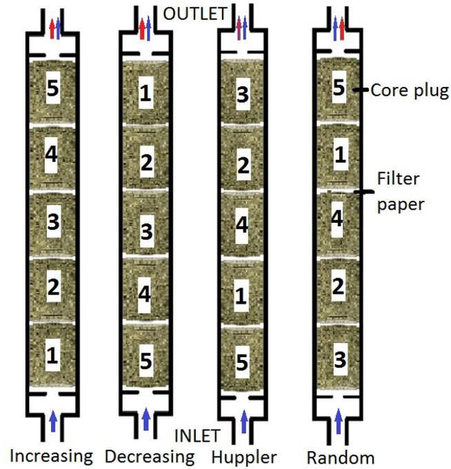
**Figure 5-6: Composite core plug arrangements (Random arrangement is only simulated, no experimental data).**
