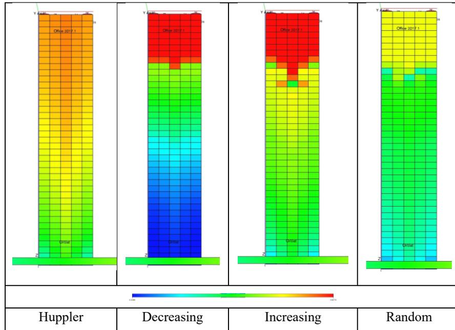
Figure 5-5: 1D 2-phase flow model with grids in Eclipse 100 ©.
