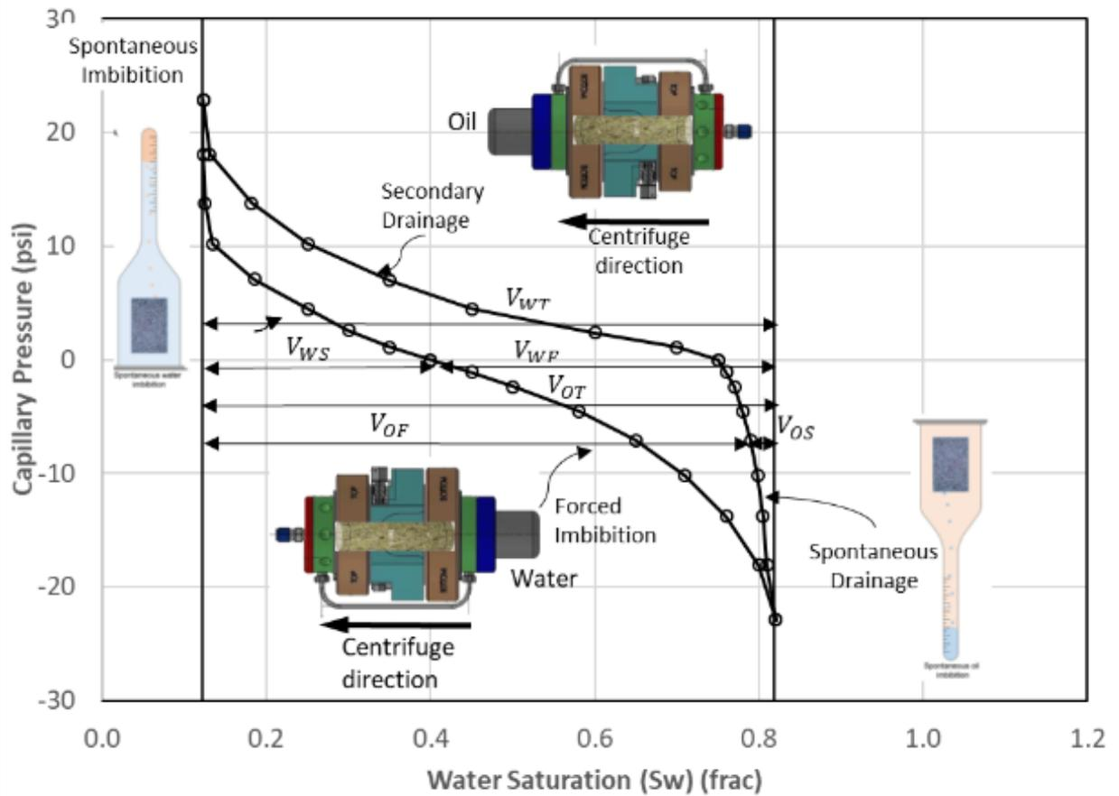
Figure 2-2: Schematic of wettability measurements throughout the Amott test
