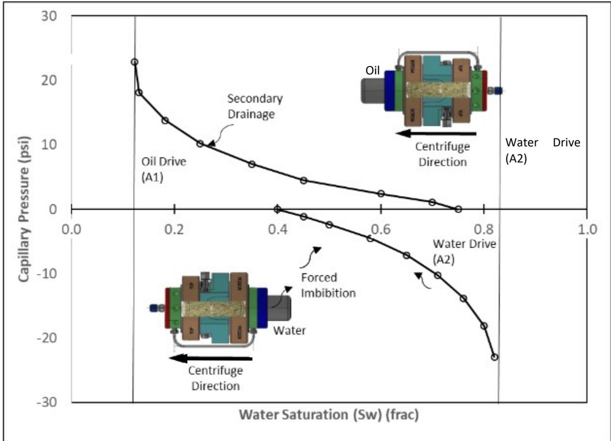
Figure 2-3: Schematic of wettability measurement by USBM method
