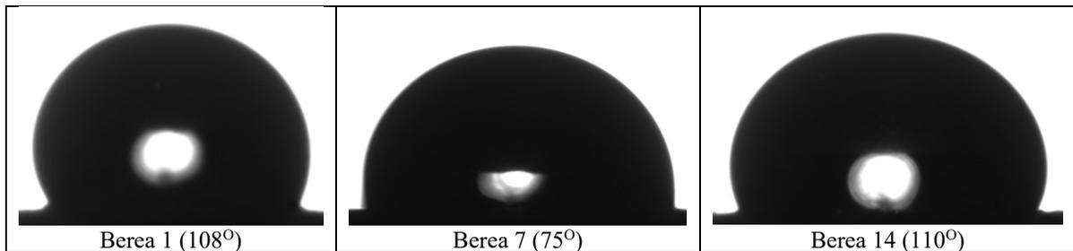
**Figure 3-1: Contact angle measurements for Berea.**
