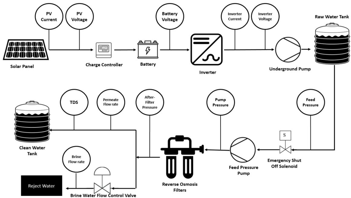
Figure 45: Complete System Process and Instrument flow Diagram
