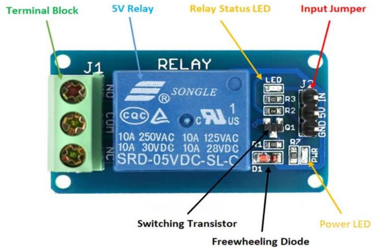
Figure 57: Relay module physical hardware and connection points [29]
