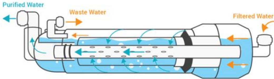
Figure 27: Water flow inside reverse osmosis membrane [30]
