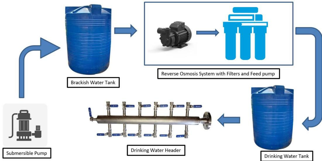
Figure 12: Water System Configuration
