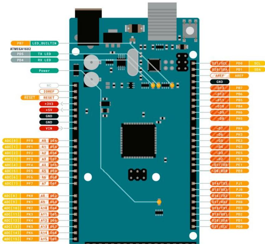
Figure 59: RTU Pin Configuration [32].
