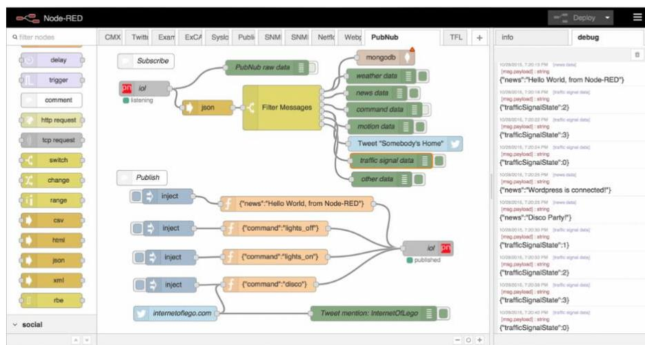
Figure 61: Node-Red web based flow programming environment [36].
