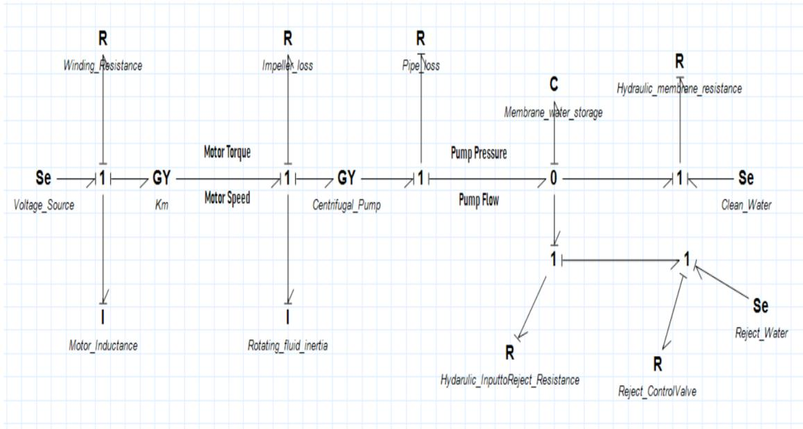
Figure 29: Complete System Bond Graph Model
