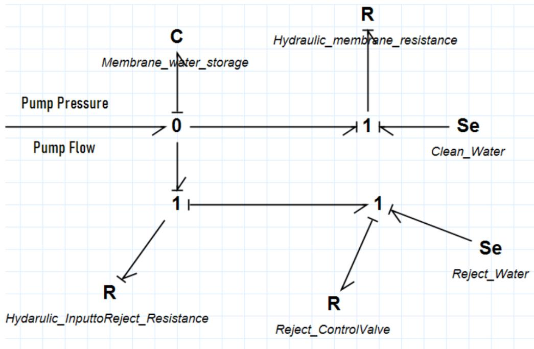
Figure 28: Bond Graph Model of Reverse Osmosis System
