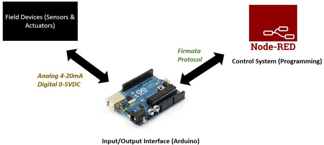
Figure 44: Block Diagram of Control and Monitoring System Implementation
