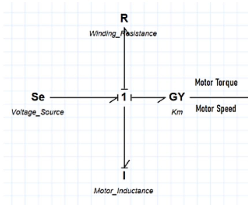
Figure 25: Bond Graph Model of Electrical System
