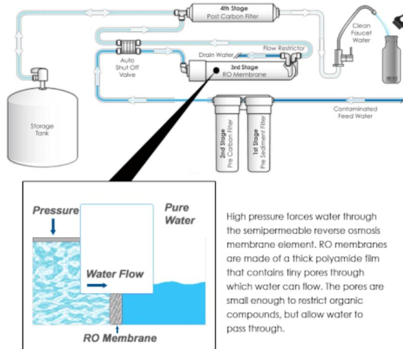
Figure 7: Reverse Osmosis Plant Flow Diagram [17]
