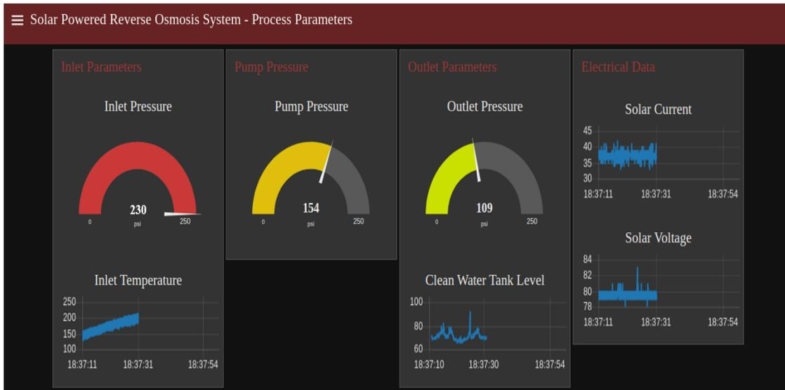
Figure 68: Node-Red Dashboard for Real-Time Monitoring.
