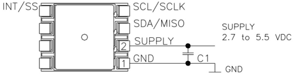
Figure 54: Pressure sensor connection diagram [26].
