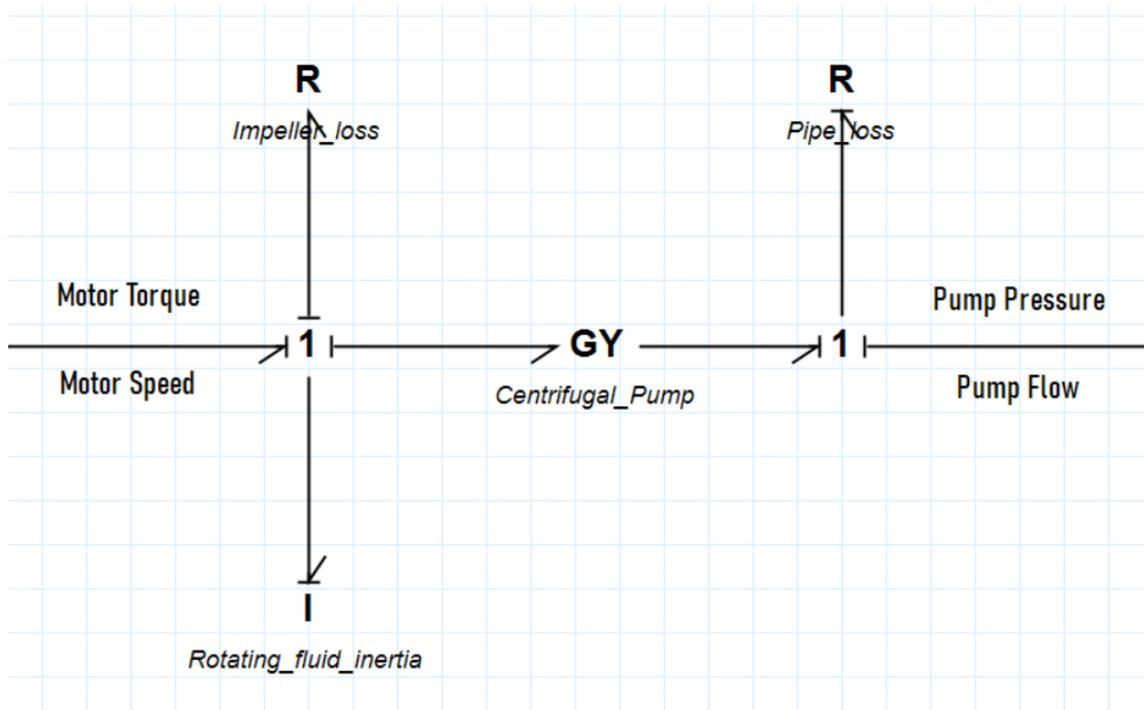
Figure 26: Bond Graph Model of Centrifugal Pump
