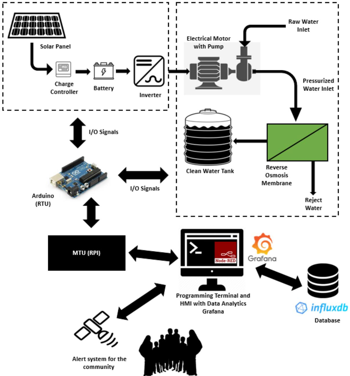
Figure 51: Proposed SCADA System for a Solar Powered Reverse Osmosis Desalination System Architecture
