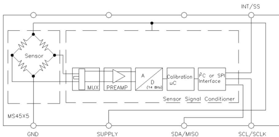
Figure 53: Pressure sensor internal block diagram [26].
