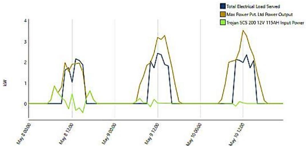
Figure 17: Comparison of total electrical load served, PV Panel Power output and battery input power
