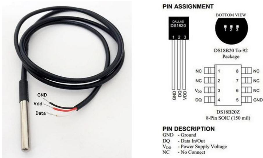
Figure 55: Temperature sensor physical and connection diagram [27].
