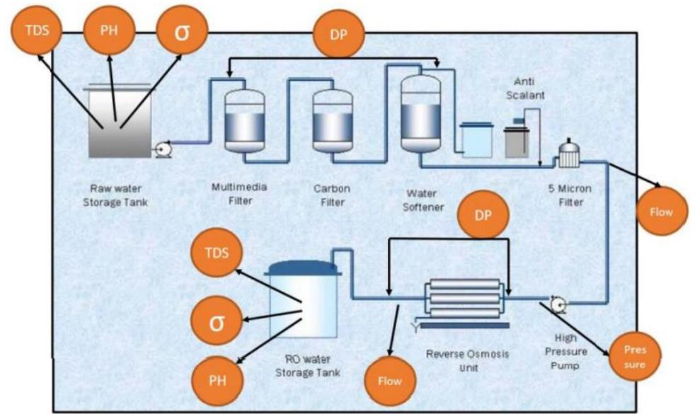
Figure 23: Block Diagram of Reverse Osmosis System
