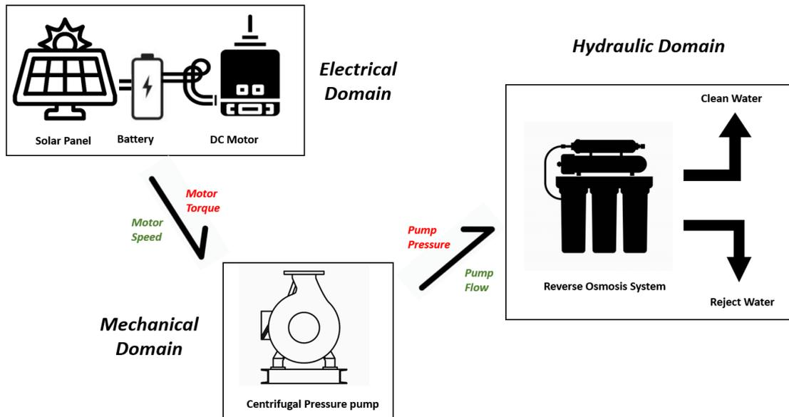
Figure 24: Generalized Bond Graph Model of System
