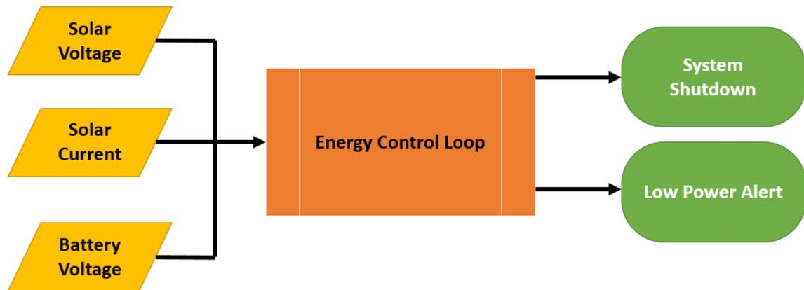
Figure 46: Energy Control Loop
