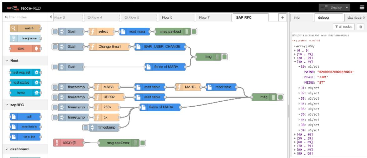
Figure 43: Browser based Programming Environment of Node Red
