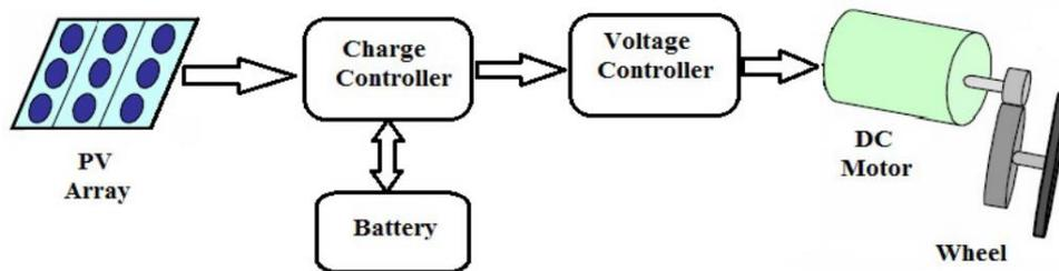
Figure 22: Block Diagram of Solar Powered DC motor [23]
