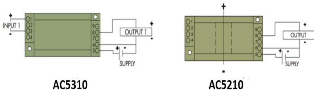
Figure 52: Current and voltage sensor wiring diagram [24, 25].
