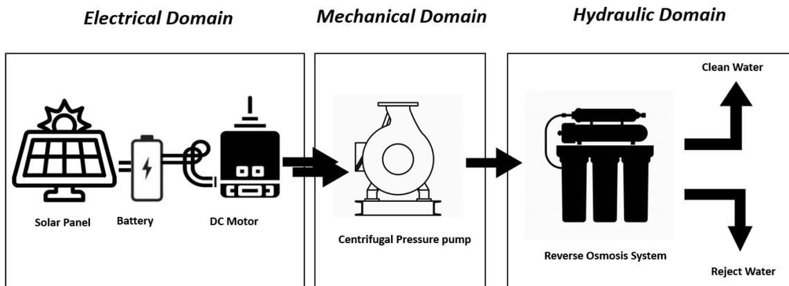
Figure 21: Block Diagram of Complete System
