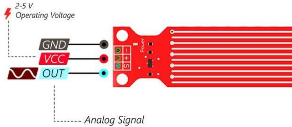
Figure 56: Water level sensor physical and connection diagram [28].
