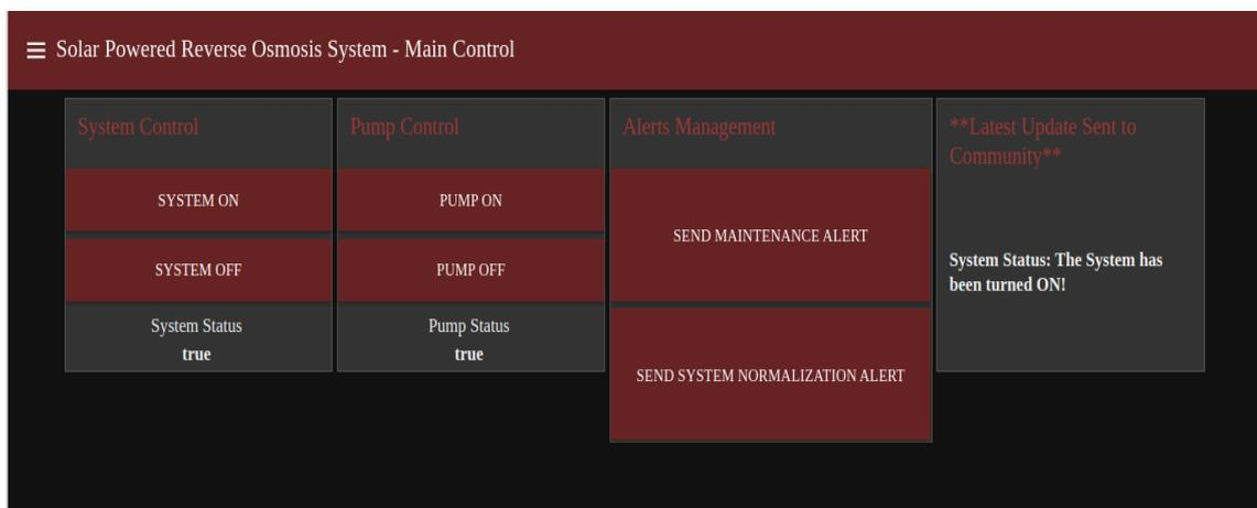
Figure 67: Node-Red Dashboard for Operation.
