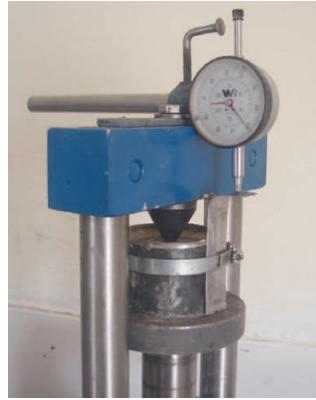
Figure 2-2 Indentation testing using metal indenter on the point load apparatus (Kahraman et al., 2012) indentation test (Kahraman et al., 2000). The DI calculation is different from the IHI: it is the slope at the 0.5 peak load on the Load/Displacement curve.
