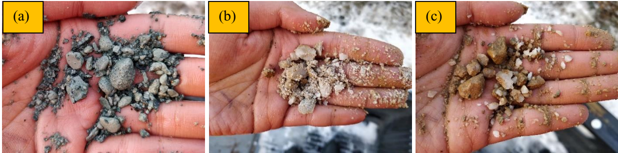
Figure 5-97 Rock cutting samples: Surrounding rock of Mafic Massive Flow (a), quartz (gold ore) (b), and a small layer of Quartz/Altered (c) for cutting analysis
