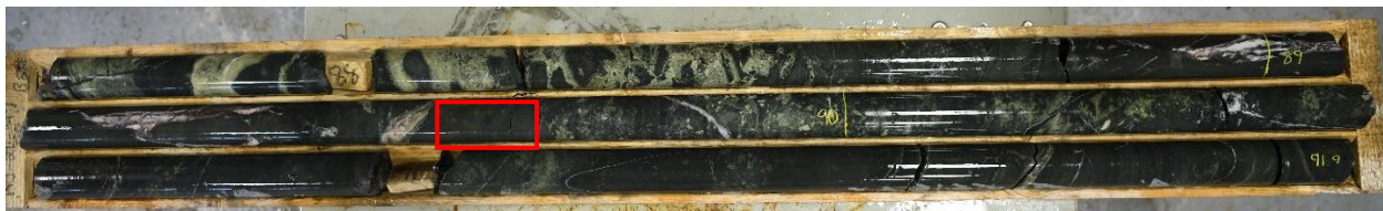
Figure 4-6 Light dark grey mafic massive flow, 87.6m-92m. Red box marks the XRD and MLA sample location.
