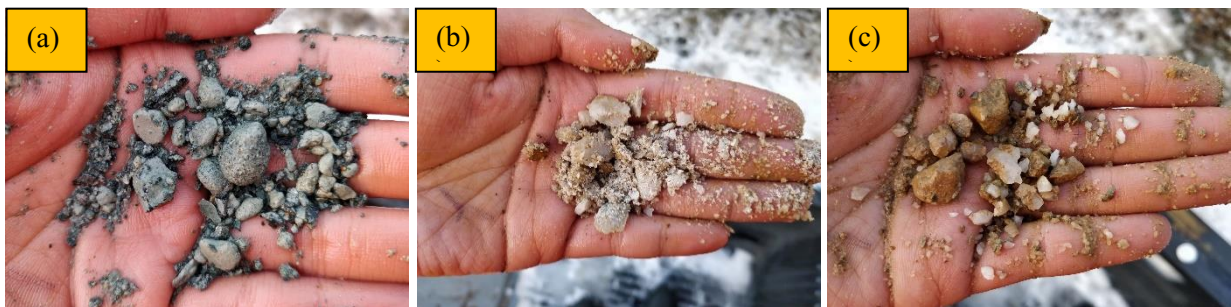
Figure 4-2 The lithology of the rock cutting samples changes with depth: Surrounding rock of Mafic Massive Flow at 2m deep (a), quartz at 4.5m deep (gold ore) (b), and a small layer of Quartz/Altered at 7m deep (c), (Li et al., 2019).
