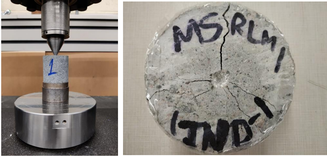
Figure 8-6 Left: the indentation test on the unstrapped rock sample. Right: Top view of crater and fracture formed on an indentation sample. The sample is tested with metal strip during the indentation test. (Premraj, et al., 2022)
