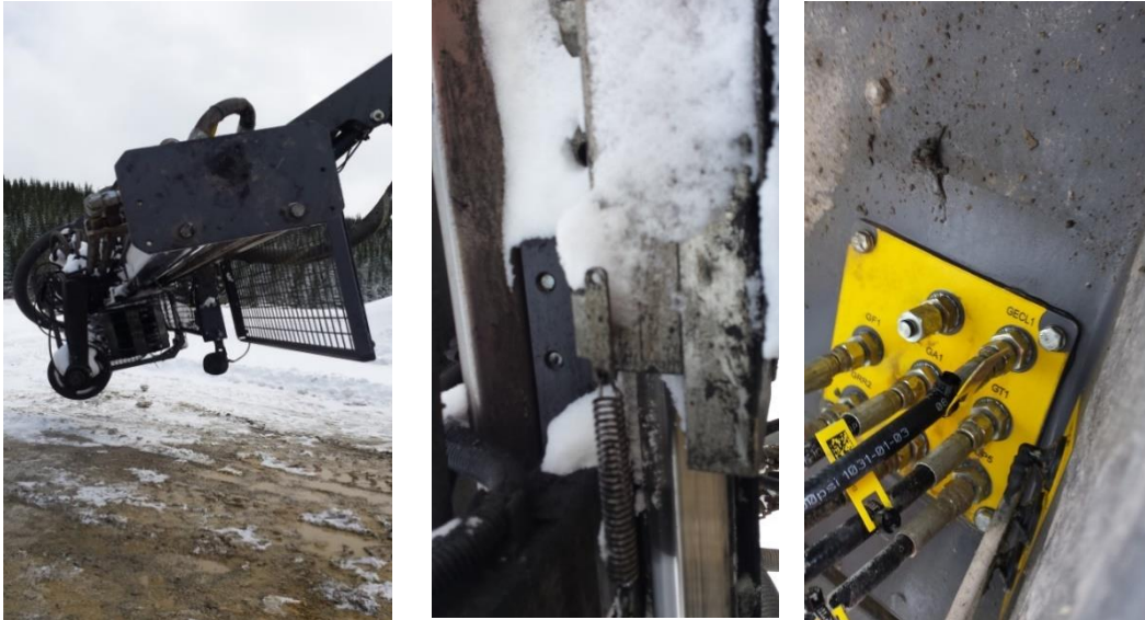
Figure 3-11 Top plate for mounting and the hose drum for cable connection, and the pressure hoses with labelling
