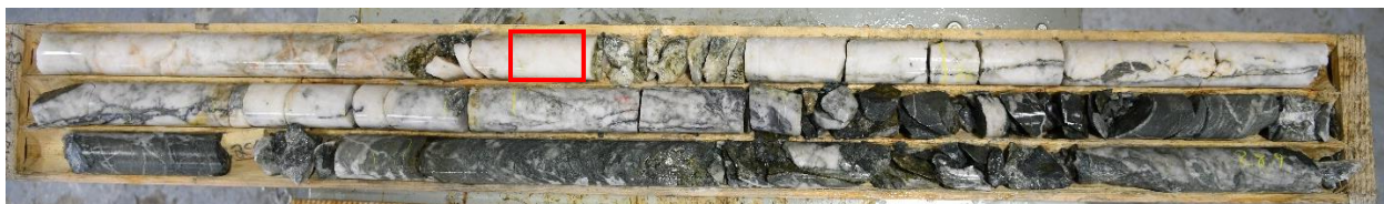
Figure 4-6 Mafic volcanic transition to massive quartz vein, 25.2m-29m. Red box marks the XRD and MLA sample location.
