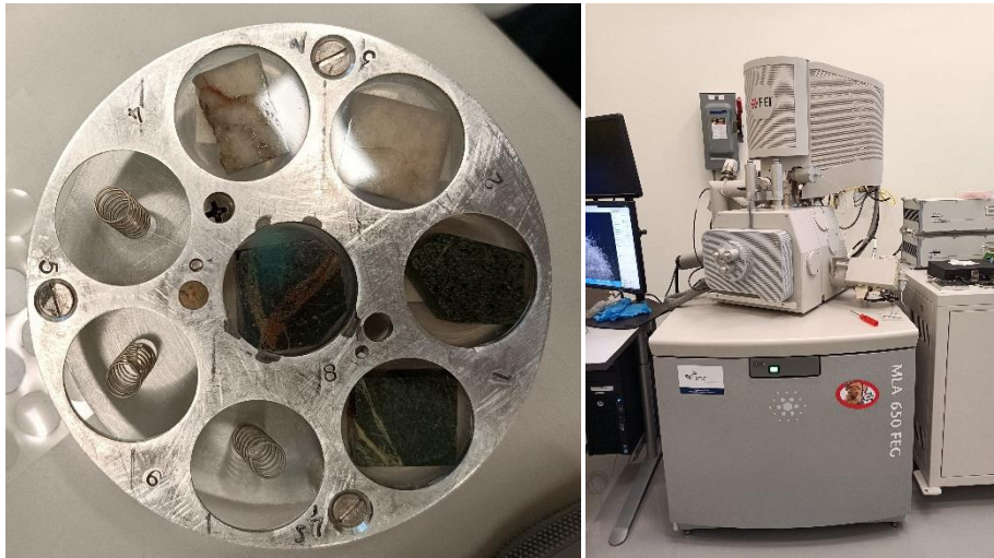
Figure 4-4 Left: Rock sample coated in epoxy mounted on the holder. Right: The MLA-SEM facility in the CREAT laboratories at Memorial University in Newfoundland
