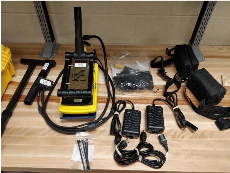
Figure 5-3 1GHz Noggin GPR unit
