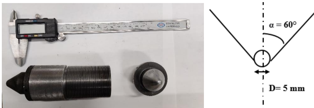
Figure 8-5 Indentation indenter. (Premraj, et al., 2022)
