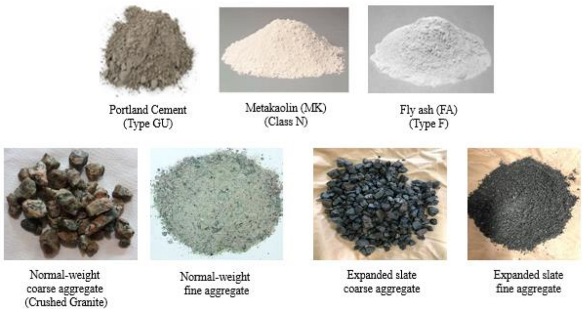
Figure 2-2: Cementitious materials and aggregates used.
