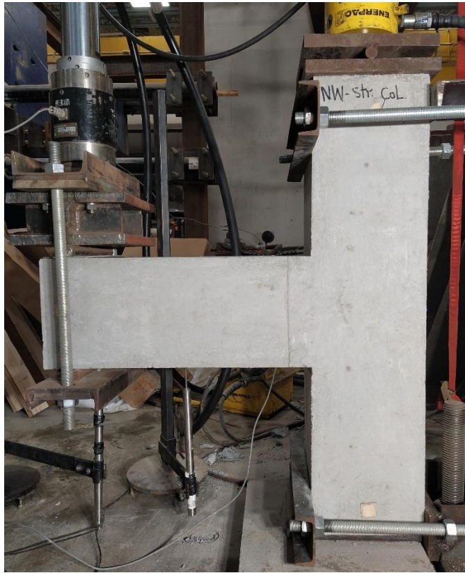
Figure 7-2: Test setup (Note: 1 mm = 0.039 in.).
