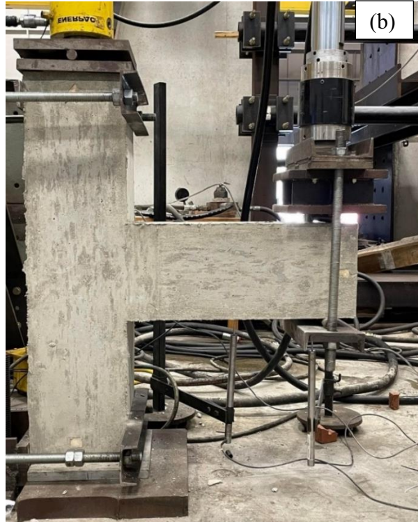
Figure 8-2: Configuration of: (a) Specimen dimensions and reinforcement details; and (b) test setup.
