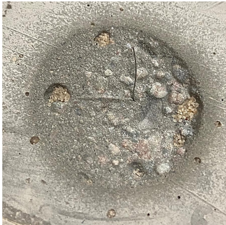
Fig. 4-22 Elemental CCSF nearly delaminated under sandblasting abrasion test.
