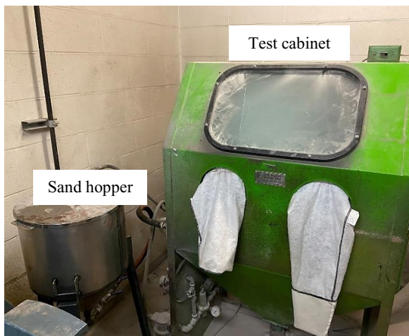
(b) Test cabinet and the sand hopper.
