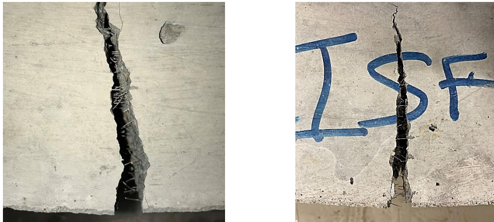
(a) Control mixture typical specimen (b) NPs incorporated typical specimen
