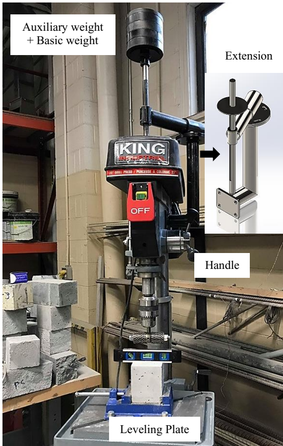
(a) Drill modification.
