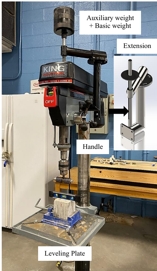
(a) Drill modification.
