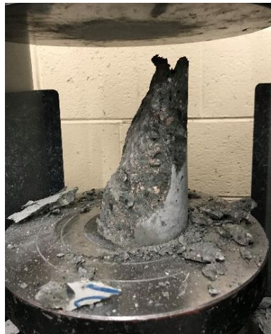
(a) Plain concrete typical specimen
