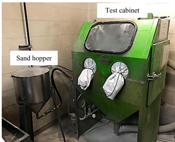
(a) Test cabinet and the sand hopper.
