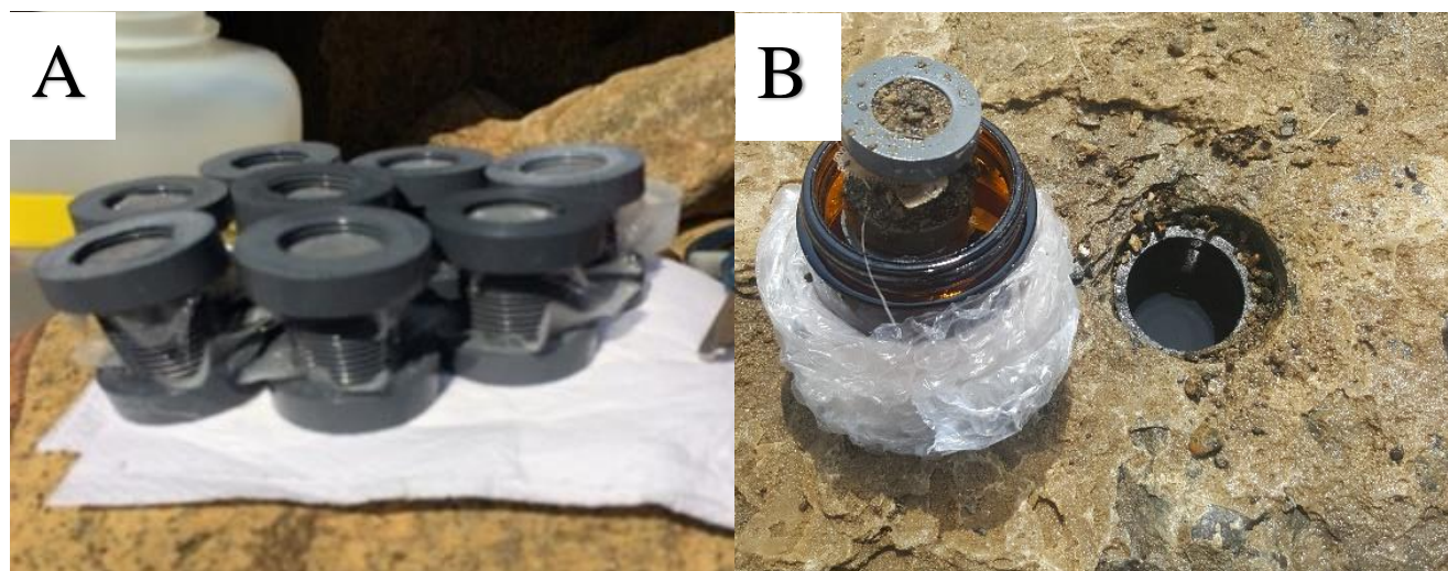
Figure 5.3. (A) The sterilized incubators and (B) the incubators after a year of exposure to the ultra-basic fluids at WHCMO.
