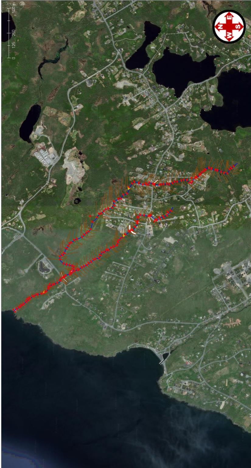
Figure A.10: Plan View of Goat River HEC-RAS model with cross sections indicated by red lines
