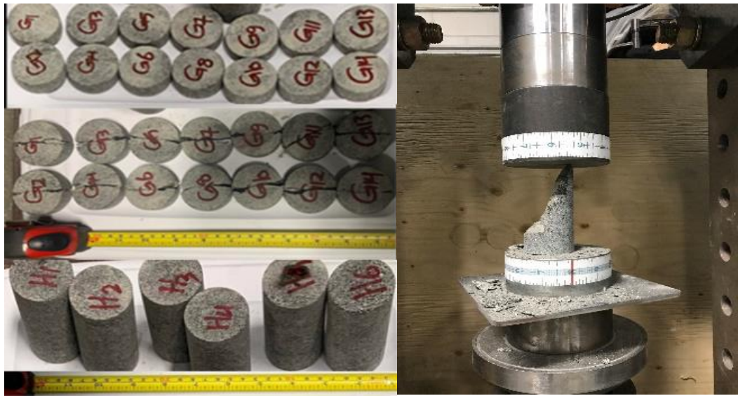
Figure 5-3. Left : (top and middle): samples for IT - before and after testing. Left : (bottom): VP, VS, and UCS samples before testing. Right: UCS sample after tests
