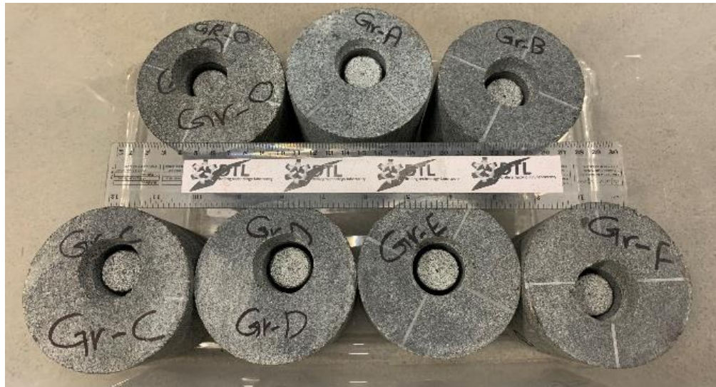
Figure 6–3. Granite sample after DOT-Test On SDS.
