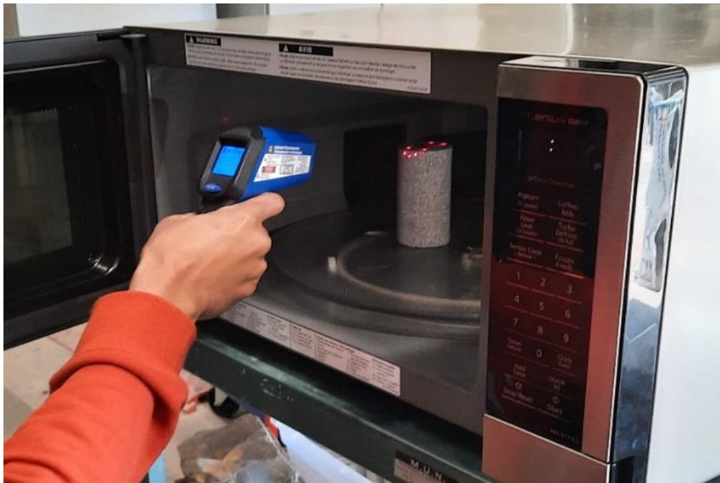
Figure 6–6. Recording temperature of the specimen by using infrared gun
