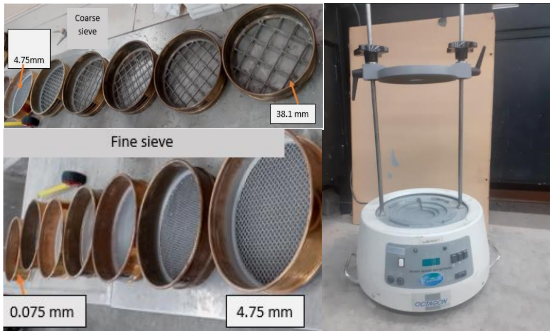
Figure 3–8. Left: Sieve set for finer and coarser and Right: Mechanical sieve shaker
