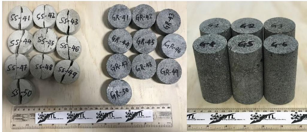
Figure 6–2. Left and Middle: Unheated-IT Samples and Right: Heated samples for Ultrasonic wave Test
