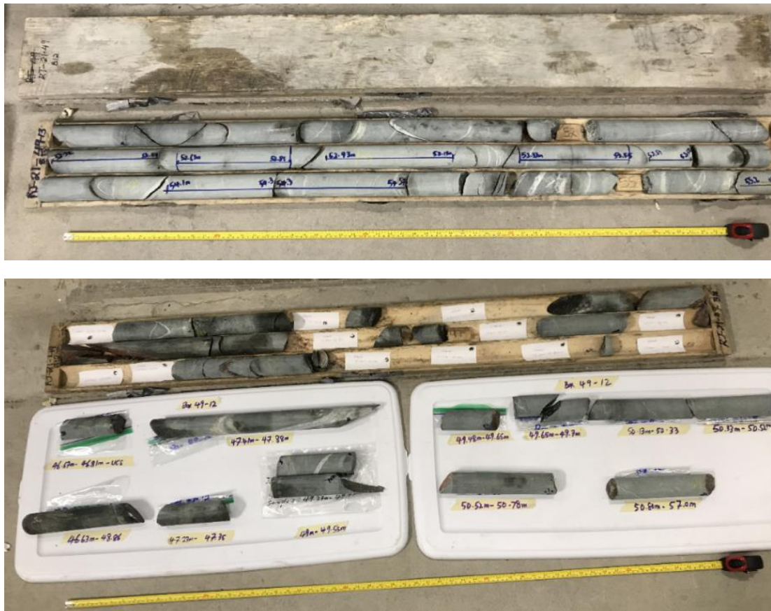
Figure 3–4. Core logging and sample selection for Laboratory test at MUN (Mafazy et al., 2022)
