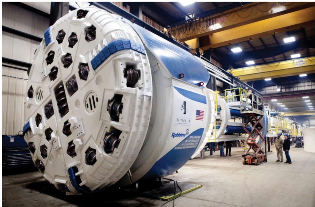
Figure 2–1. The mining head of James Robbins TBM (Krzysztof & Piotr, 2019)
