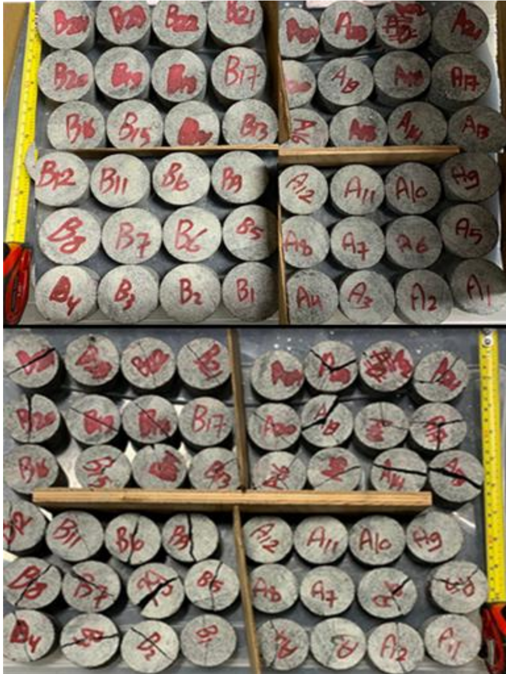
Figure 5-1. Samples for Semi-PLSI and PLSI tests (Group A and B), respectively before and after testing
