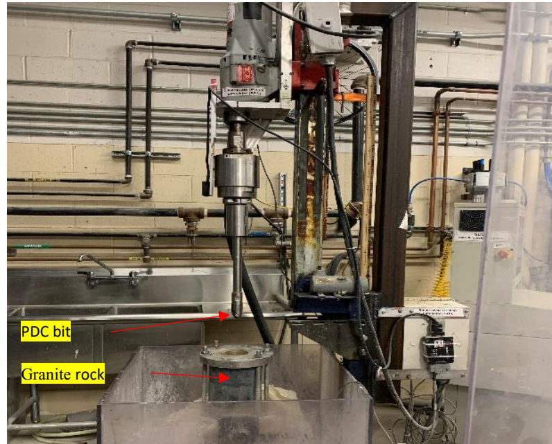
Figure 6–4. DOT Set-up on Small-Scale Drilling Simulator for the granite rock sample before and after MI.
