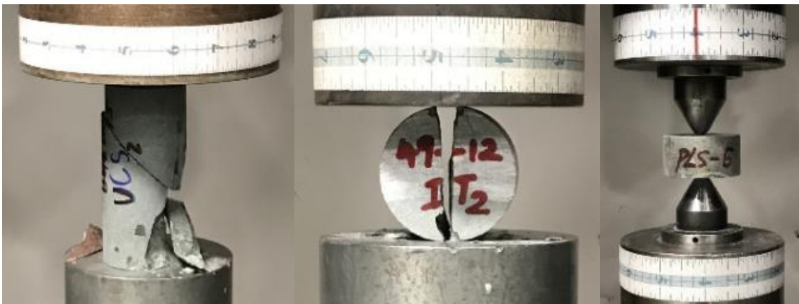
Figure 4–4. Left: UCS, Middle: ITS, and Right: PLSI; experimental setup on the geomechanics frame at Drilling Technology Laboratory (DTL), MUN
