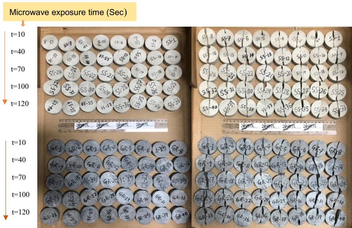
Figure 6–1. Heated Samples, Left: Before IT test and Right: After IT test
