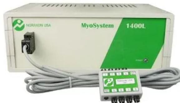
Figure 3.1: The MyoSystem 1400L EMG acquisition device.
