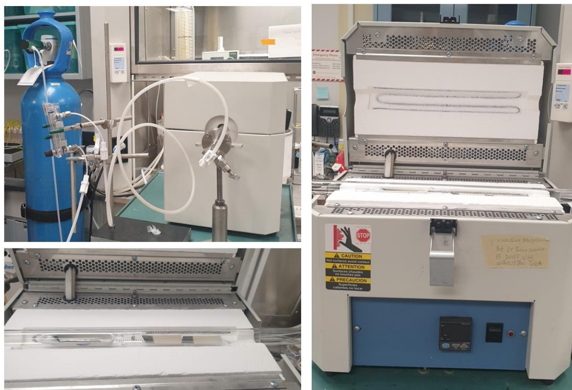
Figure 19: Sintering procedure by Electric furnaces (Lindberg/Blue M™ Moldatherm™ Box Furnaces)
