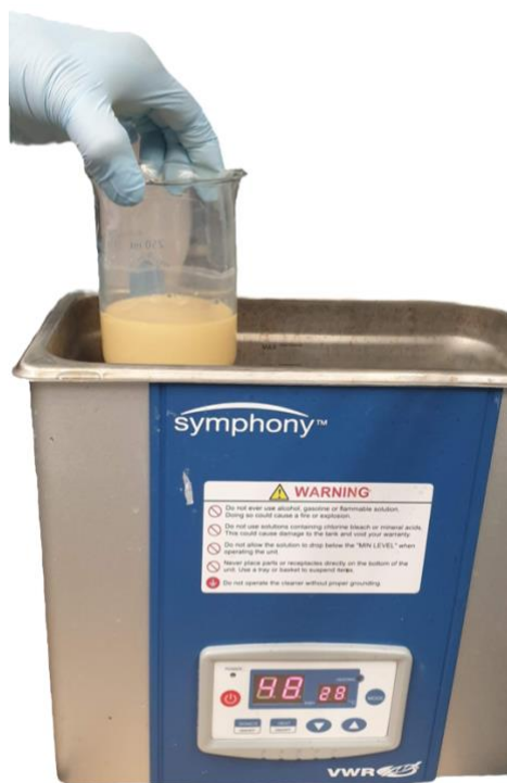
Figure 17: Preparing the coating solution by sonication stirring.
