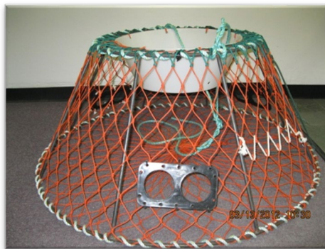
Figure 1. 8 Conical crab pot used by harvesters (Photo Courtesy of CASD, Marine Institute, MUN)
