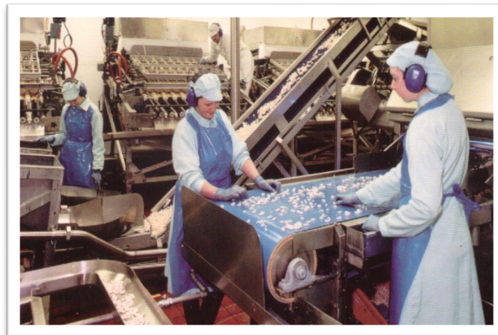
Figure 1. 5 Commercial processing of cooked and peeled shrimp (Photo Courtesy of School of Fisheries, Marine Institute, MUN)
