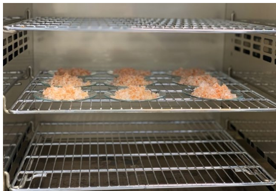
Figure 6.9 Crab shell chitin in drying oven following attempted depigmentation with hydrogen peroxide
