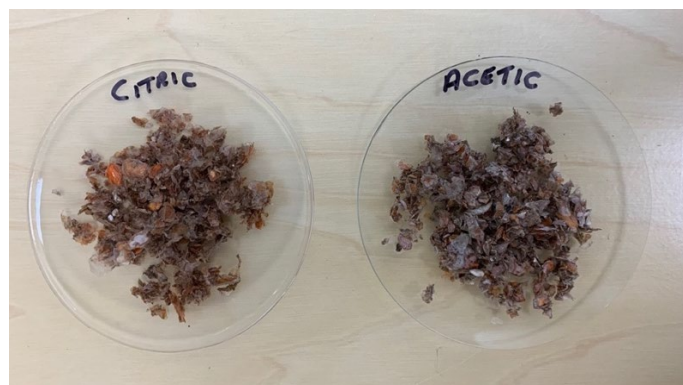
Figure 6. 7 Citric acid demineralized crab shells (left) vs acetic acid demineralized crab shells (right)
