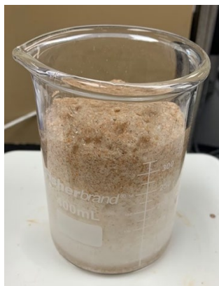
Figure 6. 8 Excessive foaming and precipitation of calcium citrate during one-step citric acid demineralization
