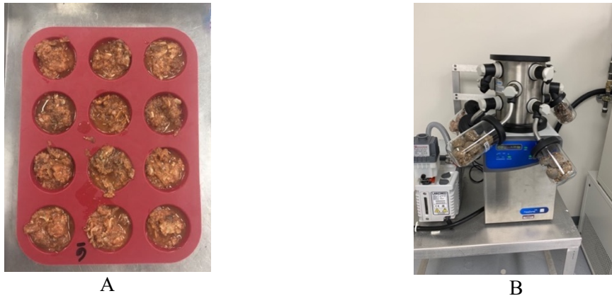
Figure 3.3 Crab feedstock samples: A - in silicon trays prior to freezing; B - in Labcono freeze drier
