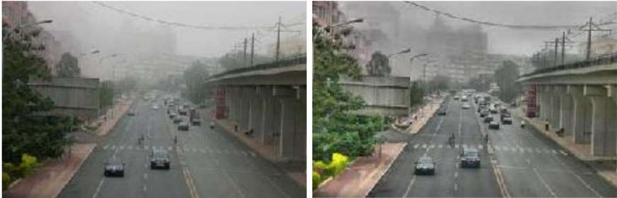
Figure 24, Foggy image before (left) and after (right) application of modified CLAHE. Adapted from figures 5 and 6 of [61].
