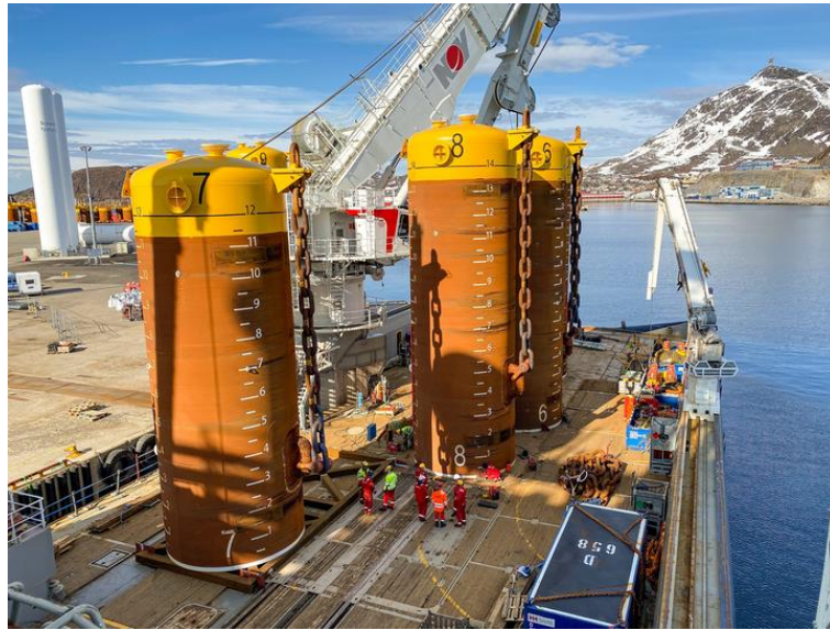
Figure 2-9. Suction anchors used with the Johan Castberg FPSO mooring system in the Barents Sea (Courtesy of Island Offshore)
