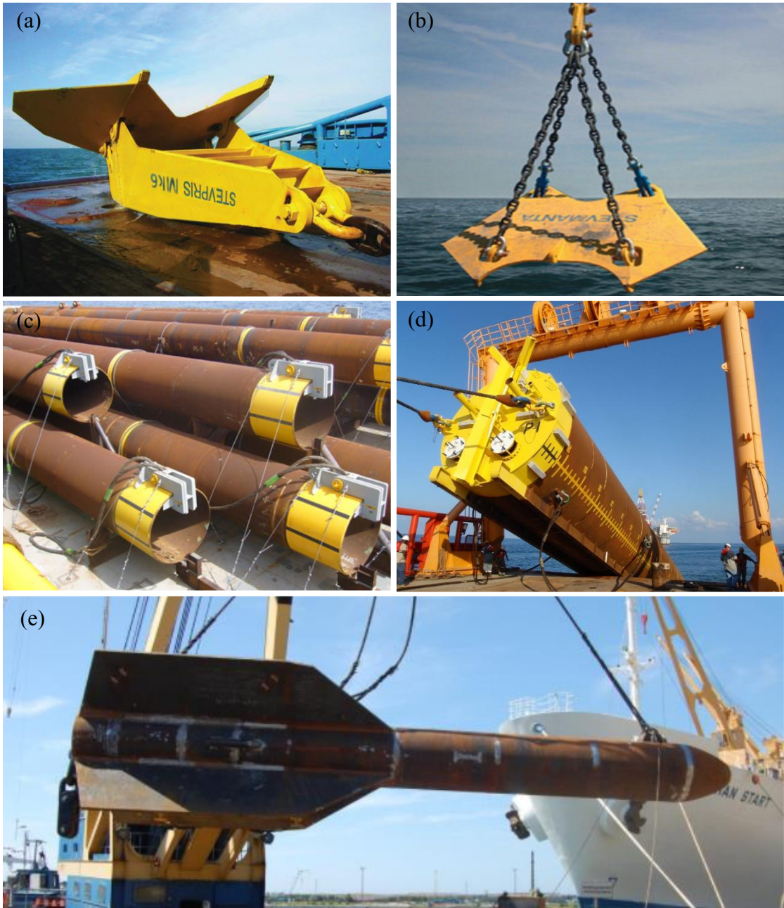
Figure 2-4. Types of marine anchors. (a) Drag embedment anchor (Courtesy of Vryhof Anchors), (b) vertically loaded anchor (Courtesy of Vryhof Anchors), (c) pile anchor (Courtesy of InterMoor), (d) suction anchor (Courtesy of InterMoor), (e) torpedo pile (Courtesy of Deep Sea Anchors)
